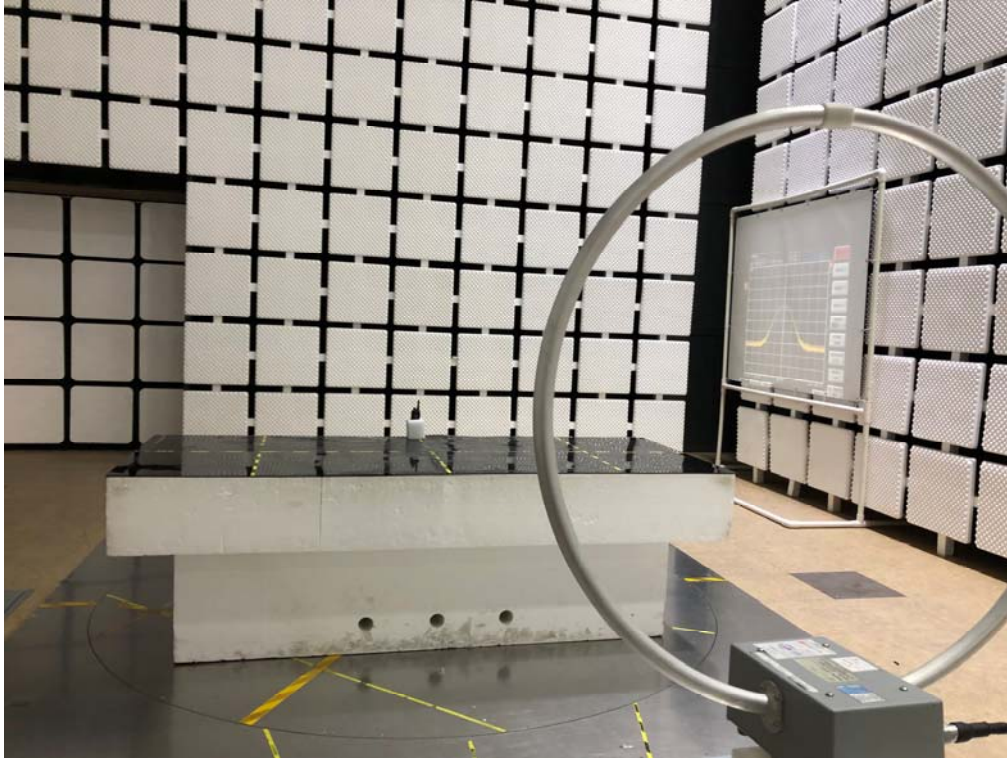
Radiated RF measurement (Below 30 MHz)
