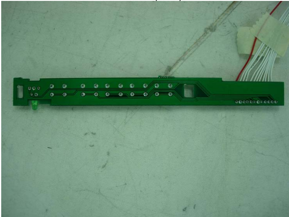
OSD Board ( Rear )
