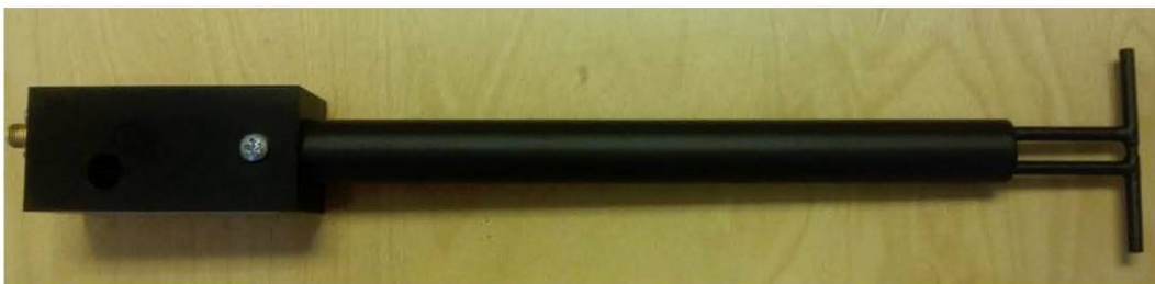
Figure 1 – MVG COMOSAR Validation Dipole
