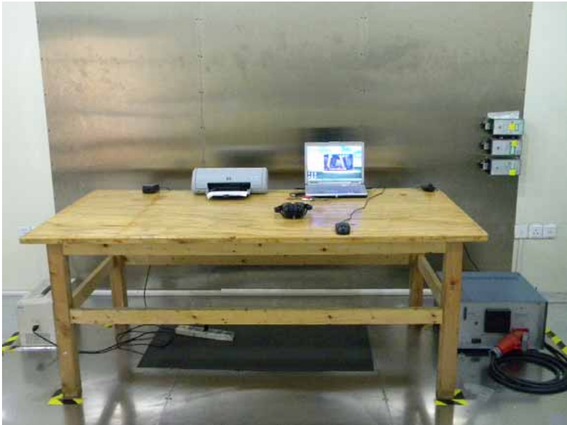
Front View of Conducted Measurement
