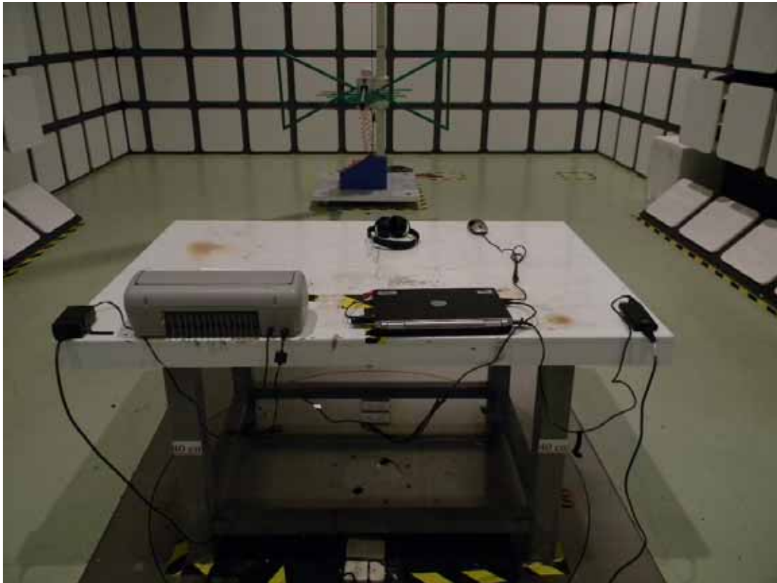
Front View of Radiated Emission Test (Working)
