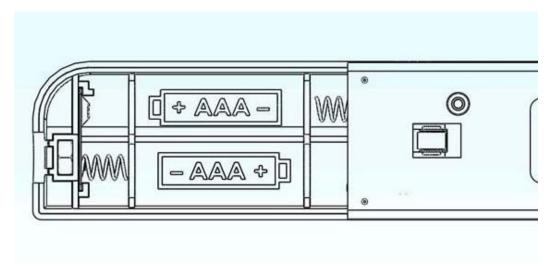
3. Slide the batter lid back on the Z-Wave Window / Door Detector and fasten the lid by using the screw.
