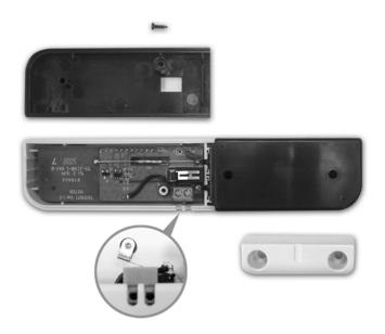
2. Now connect prepared normal switch to this two hole by screwdriver as instruction.
