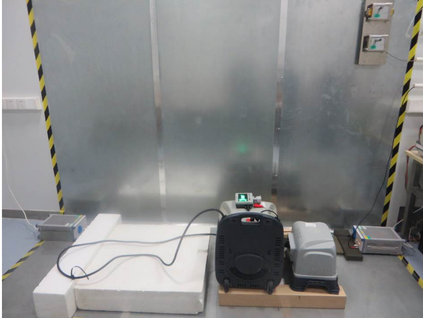
Photograph 1: Set-up for Conducted Emission Test
