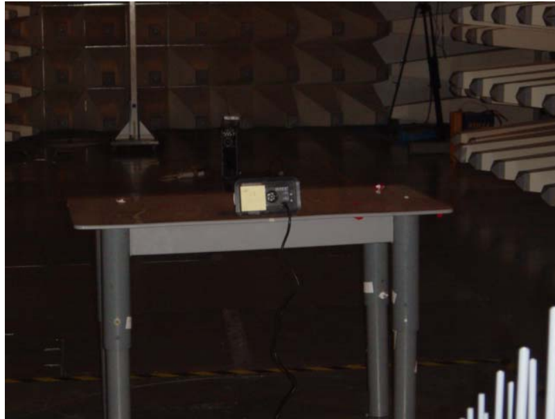
Set-up for Radiation Emission ( Receiver)
