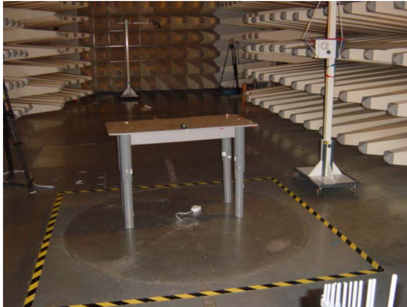
Set-up for Radiation Emission ( Transmitter)
