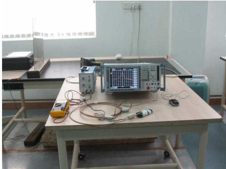
Photograph 2: Set-up for bandwidth measurement
