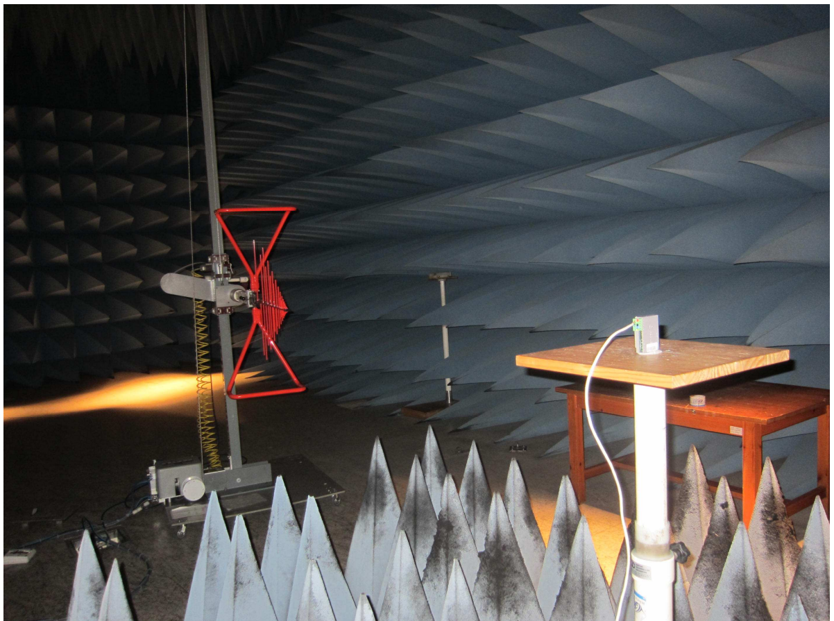
Fig. 3. Test set-up for radiated measurements above 30 MHz to 1 GHz
