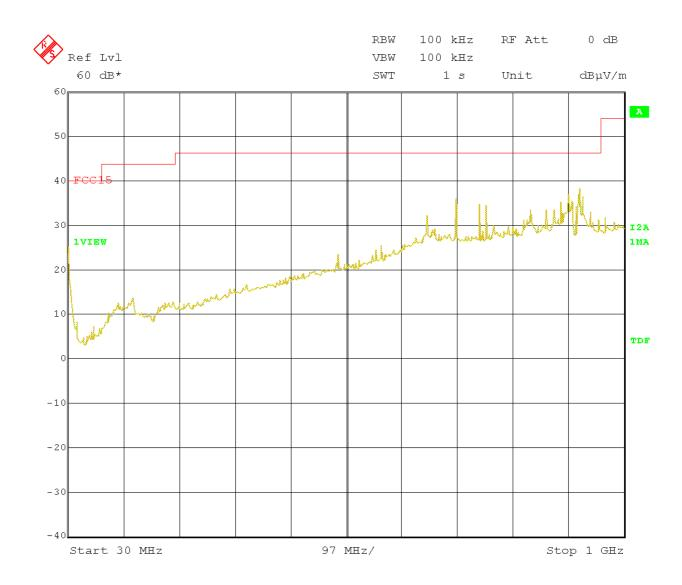
Note: The carrier is suppressed using a tuneable notch filter.
