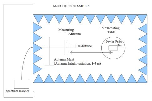
Shielded Control Room For Radiated Measurements
