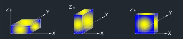
Note 1: For all radiated test, EUT in each of three orthogonal axis emissions had been tested, but only the worst case (X axis) data recorded in the report.
