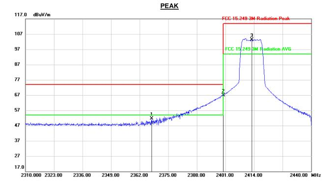
Result No. Frequency Reading Correct Limit Margin Remark (dBuV) (dB/m) (dBuV/m) (dBuV/m) (MHz) (dB)1 2367.557 18.17 33.40 51.57 74.00 -22.43 peak 2 33.17 33.82 74.00 -7.01 2400.000 66.99 peak 3 2413.000 70.24 33.10 103.34 114.00 -10.66 peak
