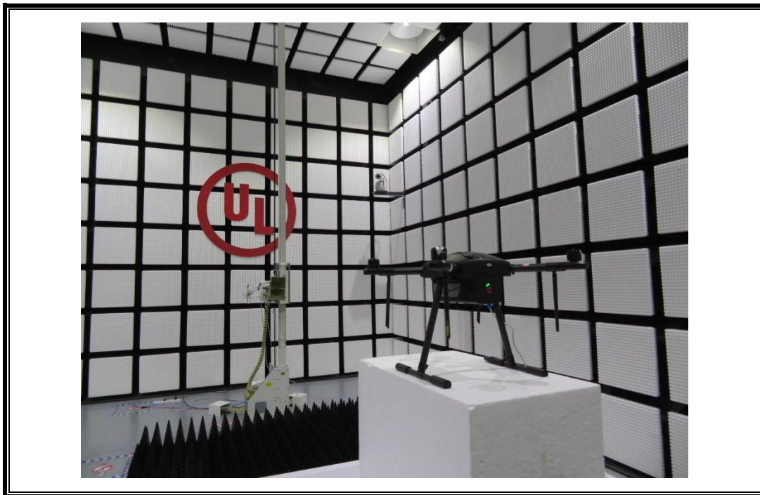
RADIATED RF MEASUREMENT SETUP (ABOVE 1 GHz- Z axis)
