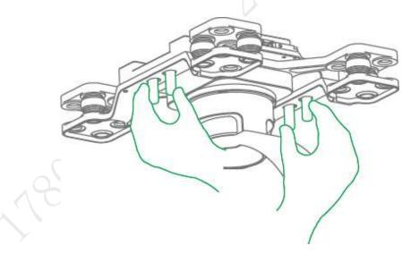
Figure 5-6 Step 2 PTZ camera is separated from the aircraft, so it is dismantled quickly.
