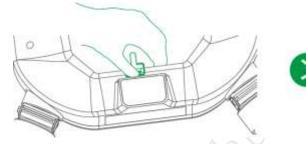
Step 1 Open silicone cover of USB port of the aircraft.
