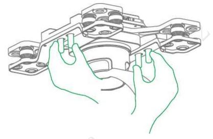
Figure 3-9 Step 2 PTZ camera is separated from the aircraft, so it is dismantled quickly.
