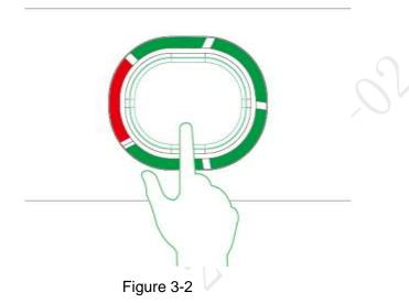
Battery switch has 5 indicator light states. The front red indicator light means that the battery is on, whereas the other 4 green indicator lights represent remaining power of the battery.
