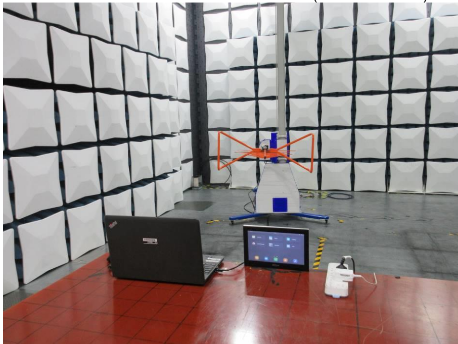
RADIATED RF MEASUREMENT SETUP (30MHz ~ 1 GHz)
