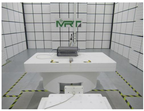
Description: Radiated Emission Test Setup for 50GHz ~75GHz (at 1m)
