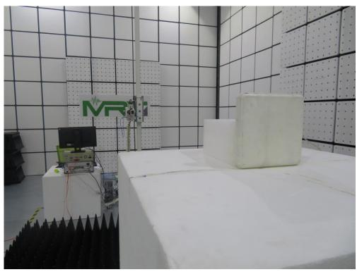
Description: Radiated Emission Test Setup for 18GHz ~40GHz (at 3m)
