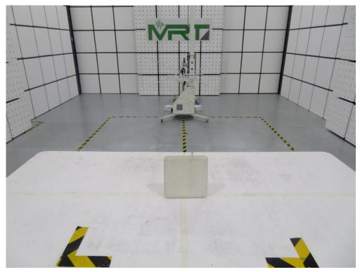
Description: Radiated Emission Test Setup for Below 1GHz (at 3m)
