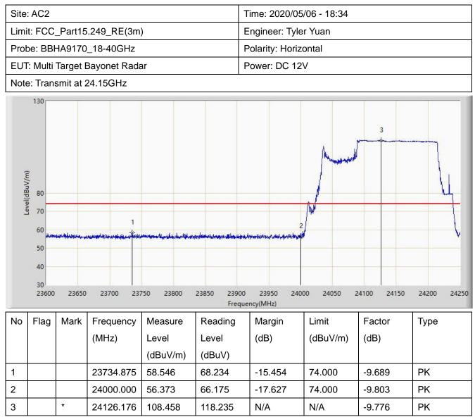
Note: Peak Measure Level  $(dB\mu V/m)$  = Reading Level  $(dB\mu V)$  + Factor (dB)
