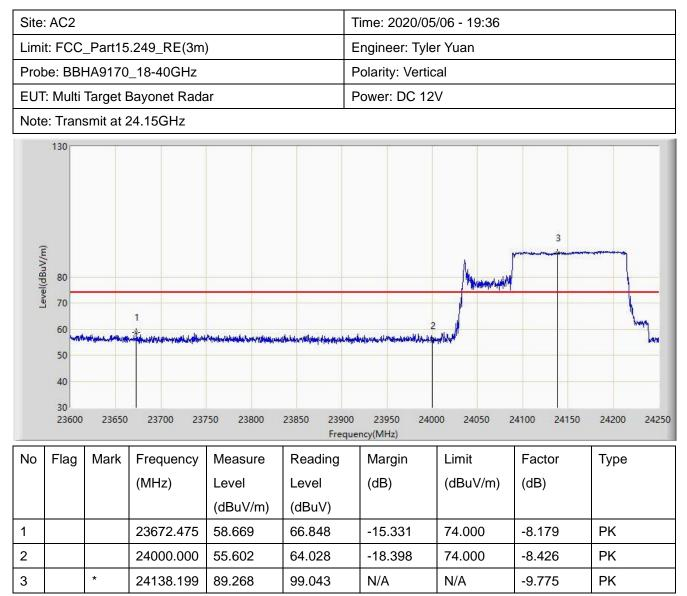
Note: Peak Measure Level (dBµV/m) = Reading Level (dBµV) + Factor (dB)
