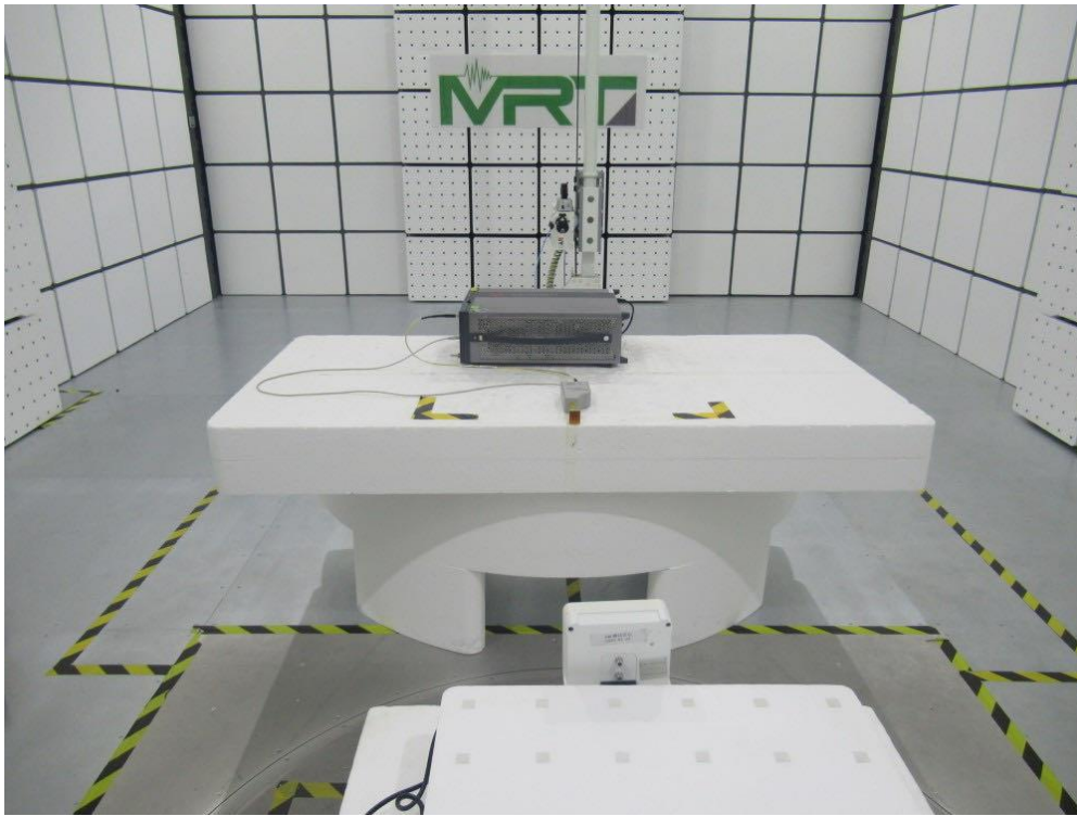
Description: Radiated Emission Test Setup for 75GHz ~100GHz (at 0.25m)
