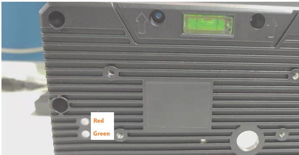
Figure 3-10 Indicator lights on the Radar
