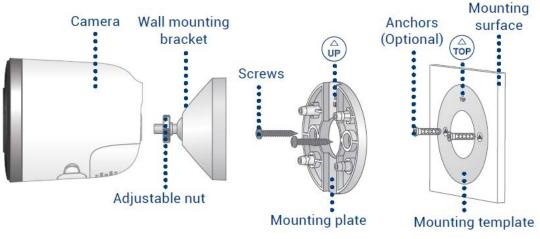
1. Place the mounting template onto the desired location.
