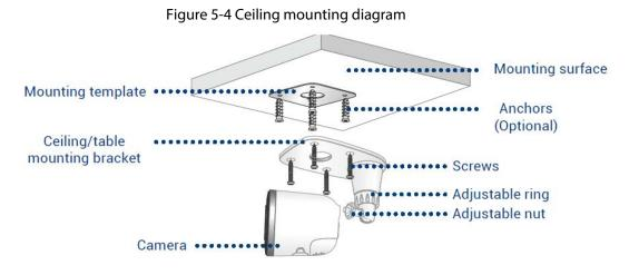
1. Place the mounting template onto the desired location.
