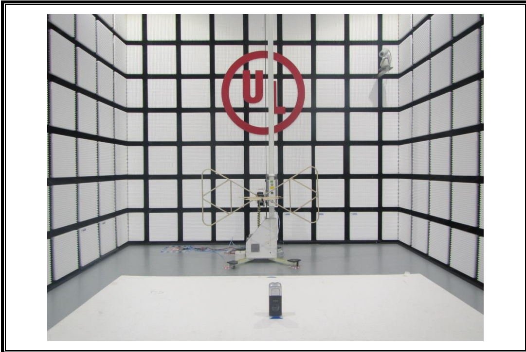
RADIATED RF MEASUREMENT SETUP (30MHz ~ 1 GHz)
