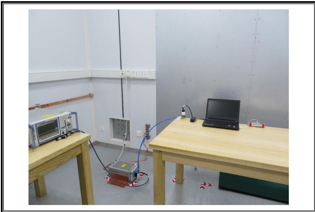
POWERLINE CONDUCTED EMISSIONS MEASUREMENT SETUP
