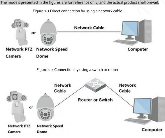
All devices have the same IP address (192.168.1.108 by default) when they are delivered out of factory. To make the Device get access to network smoothly, plan available IP segment reasonably according to practical network environment.
