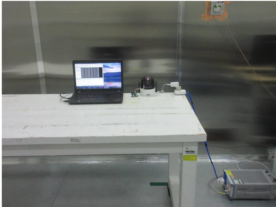
POWERLINE CONDUCTED EMISSIONS MEASUREMENT SETUP
