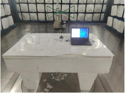
**RF Radiated Test(1-18GHz)**
