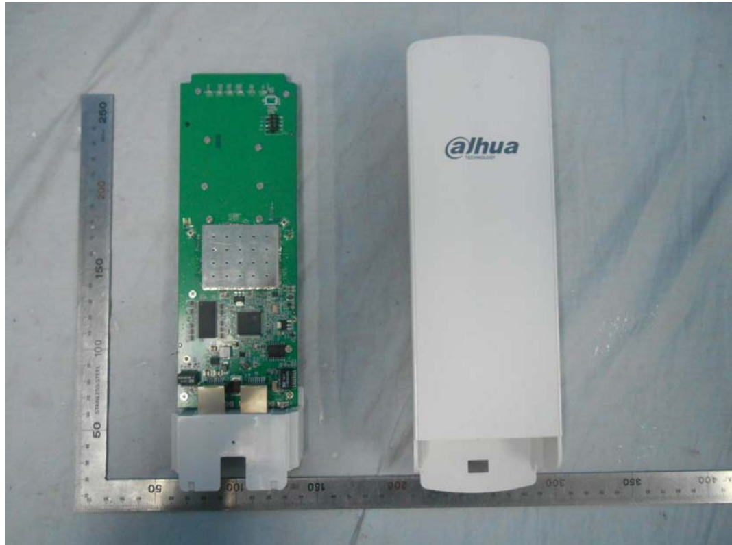
FIGURE 4 CPE (M/N: DH-PFM881) GENERAL APPEARANCE (COVER REMOVED)
