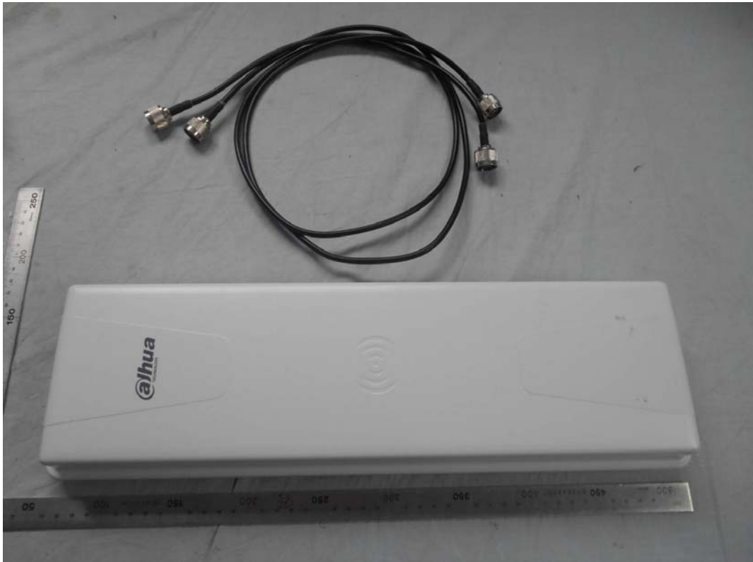
FIGURE 11 AP (M/N: DH-PFM880) ANTENNA (FRONT VIEW)
