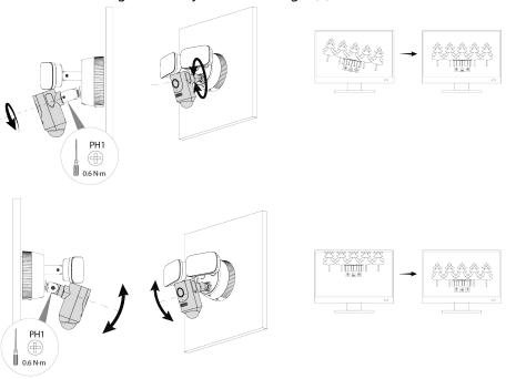
• Adjust the lens angle by rotating the universal joint only.
