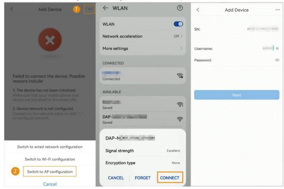
Figure 3-2 Configure the device hotspot
