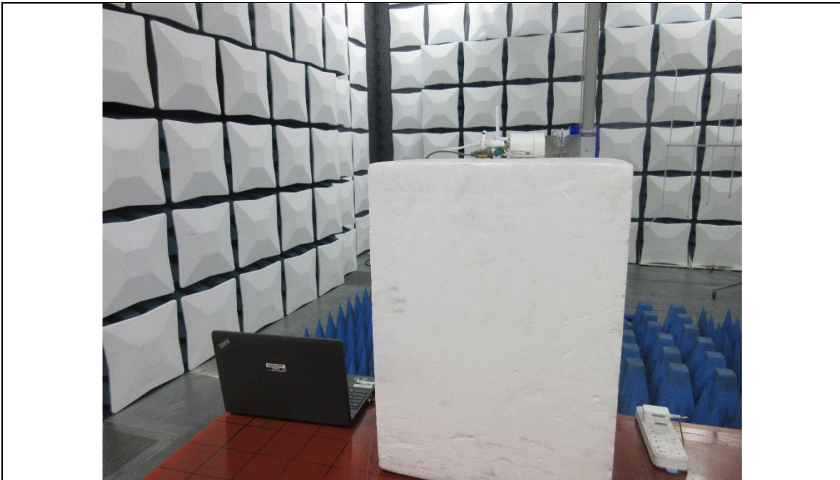
RADIATED RF MEASUREMENT SETUP (ABOVE 1 GHz- Y axis)
