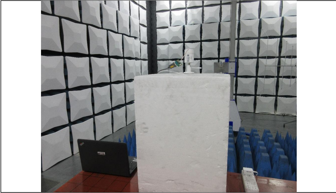
RADIATED RF MEASUREMENT SETUP (ABOVE 1 GHz- Z axis)
