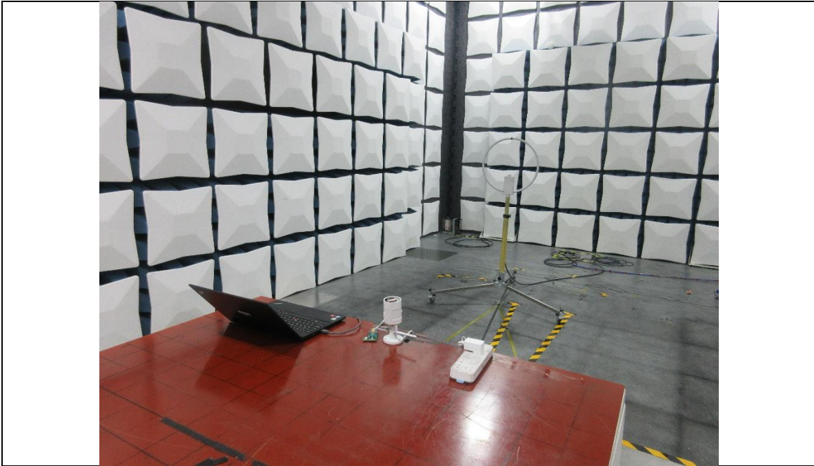
RADIATED RF MEASUREMENT SETUP (Below 30MHz)
