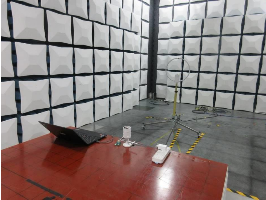
RADIATED RF MEASUREMENT SETUP (9KHz ~ 30 MHz)
