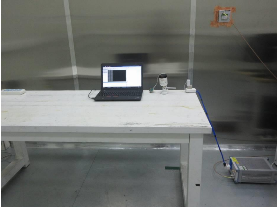
POWERLINE CONDUCTED EMISSIONS MEASUREMENT SETUP
