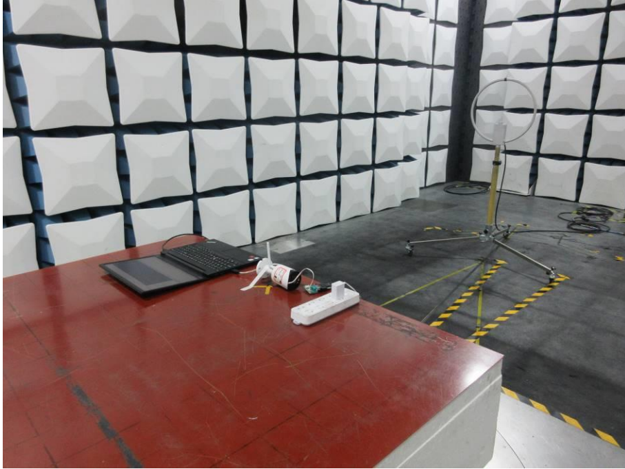
RADIATED RF MEASUREMENT SETUP (9KHz ~ 30 MHz)
