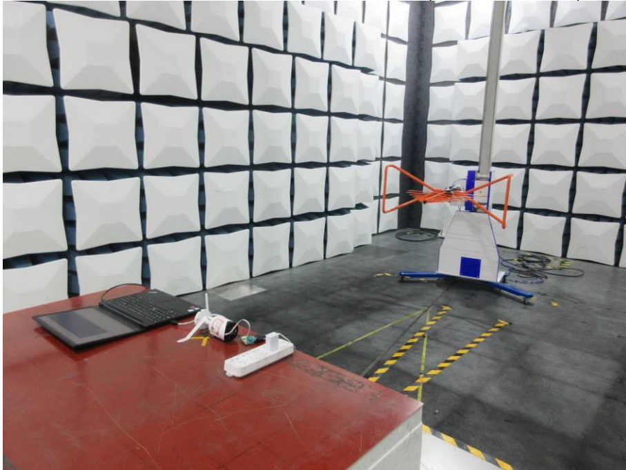
RADIATED RF MEASUREMENT SETUP (30MHz ~ 1 GHz)
