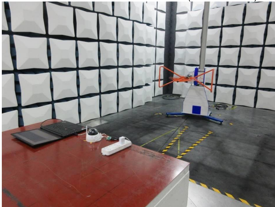
RADIATED RF MEASUREMENT SETUP (30MHz ~ 1 GHz)
