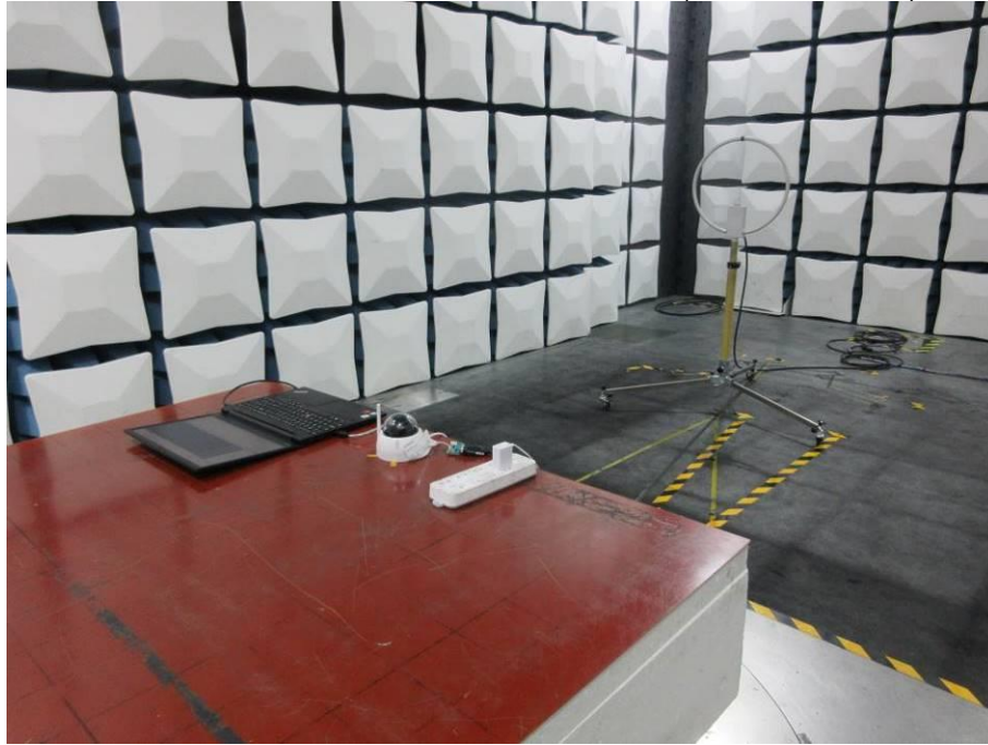
RADIATED RF MEASUREMENT SETUP (9kHz ~ 30 MHz)
