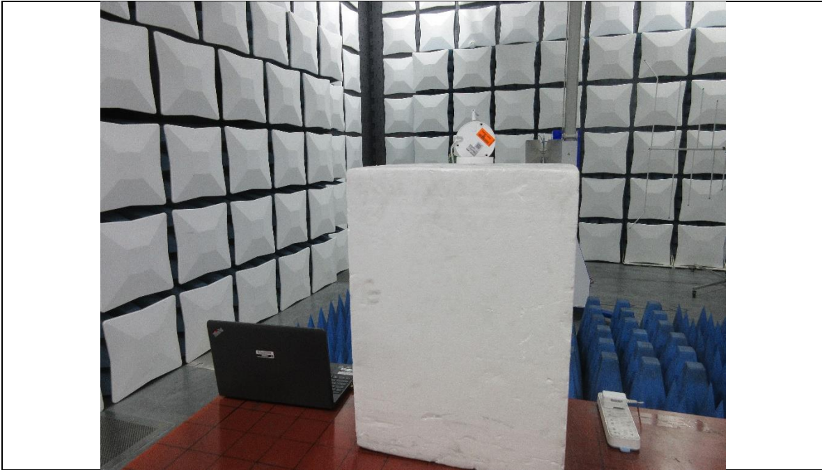
RADIATED RF MEASUREMENT SETUP (ABOVE 1 GHz- X axis)
