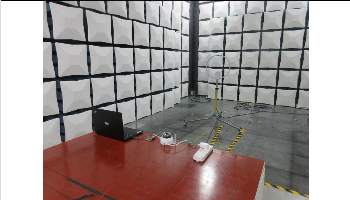
RADIATED RF MEASUREMENT SETUP (Below 30MHz)
