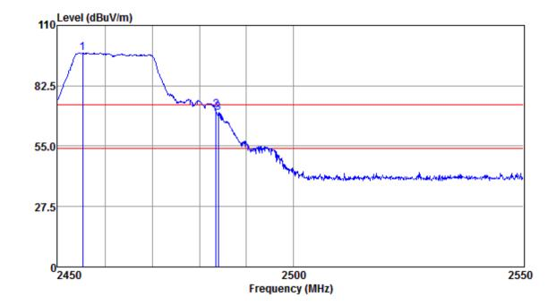
Mode:b; Polarization:Vertical; Modulation:n; bandwidth:20MHz; Channel:High
