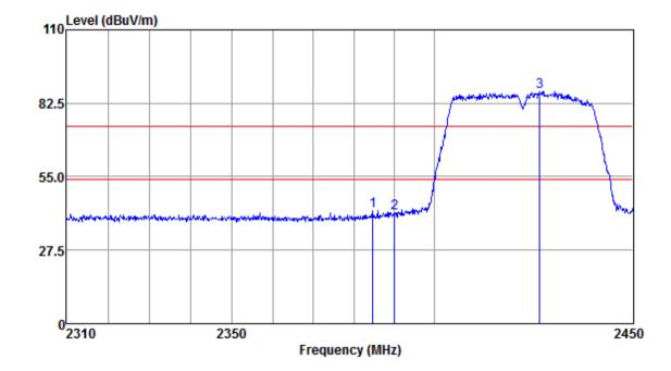
Mode:b; Polarization:Horizontal; Modulation:n; bandwidth:40MHz; Channel:Low
