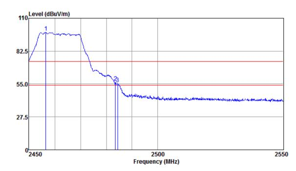
Mode:b; Polarization:Vertical; Modulation:g; bandwidth:20MHz; Channel:High
