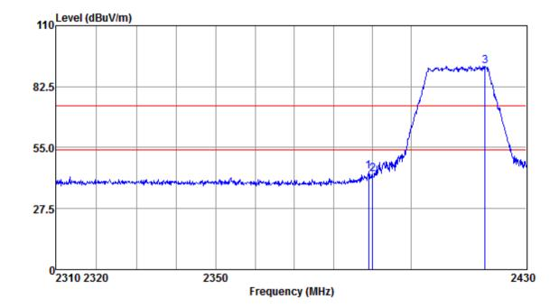
Mode:b; Polarization:Horizontal; Modulation:g; bandwidth:20MHz; Channel:Low
