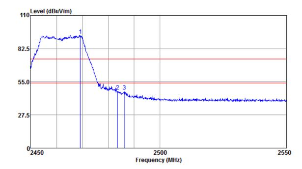
Mode:b; Polarization:Horizontal; Modulation:g; bandwidth:20MHz; Channel:High
