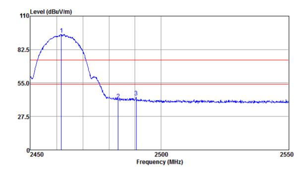
Mode:b; Polarization:Horizontal; Modulation:b; bandwidth:20MHz; Channel:High
