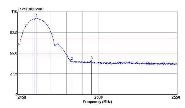
Mode:b; Polarization:Vertical; Modulation:b; bandwidth:20MHz; Channel:High
