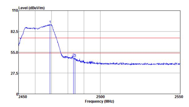
Mode:b; Polarization:Horizontal; Modulation:n; bandwidth:20MHz; Channel:High
