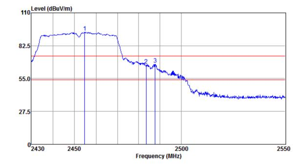
Mode:b; Polarization:Vertical; Modulation:n; bandwidth:40MHz; Channel:High
