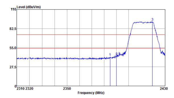
Mode:b; Polarization:Horizontal; Modulation:n; bandwidth:20MHz; Channel:Low
