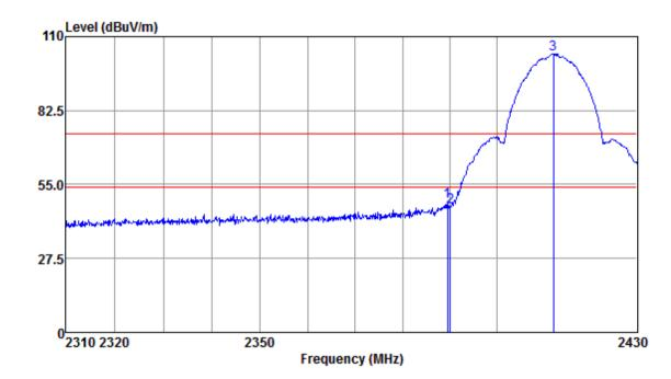
Mode:b; Polarization:Vertical; Modulation:b; bandwidth:20MHz; Channel:Low
