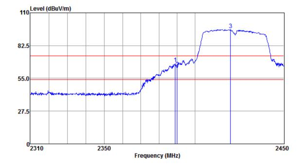
Mode:b; Polarization:Vertical; Modulation:n; bandwidth:40MHz; Channel:Low
