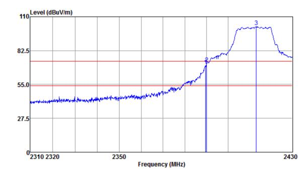
Mode:b; Polarization:Vertical; Modulation:g; bandwidth:20MHz; Channel:Low
