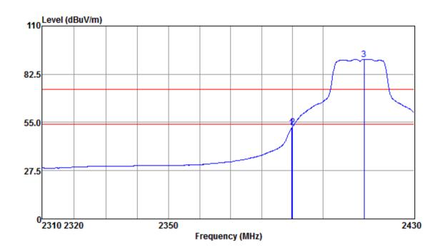
Mode:b; Polarization:Vertical; Modulation:g; bandwidth:20MHz; Channel:Low
