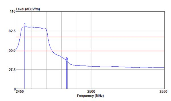
Mode:b; Polarization:Vertical; Modulation:g; bandwidth:20MHz; Channel:High
