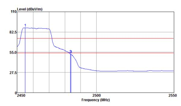
Mode:b; Polarization:Vertical; Modulation:n; bandwidth:20MHz; Channel:High
