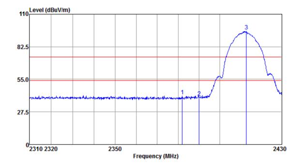
Mode:b; Polarization:Horizontal; Modulation:b; bandwidth:20MHz; Channel:Low
