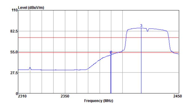
Mode:b; Polarization:Vertical; Modulation:n; bandwidth:40MHz; Channel:Low
