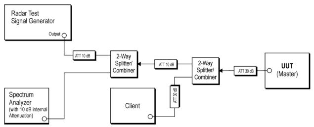
Remark: During the test, a lower radar signal level -59.69dBm was used.
