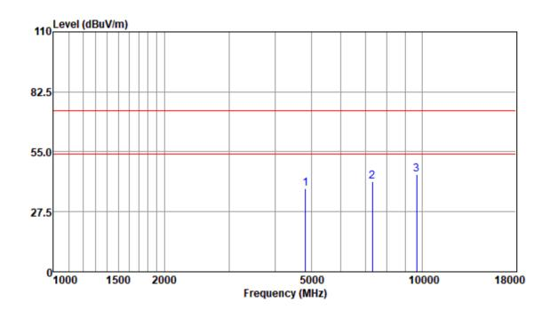
Mode:a; Polarization:Horizontal; Modulation:n; bandwidth:40MHz; Channel:Low
