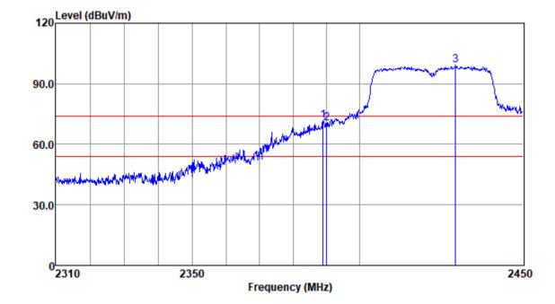
Mode:a; Polarization:Horizontal; Modulation:n; bandwidth:40MHz; Channel:Low
