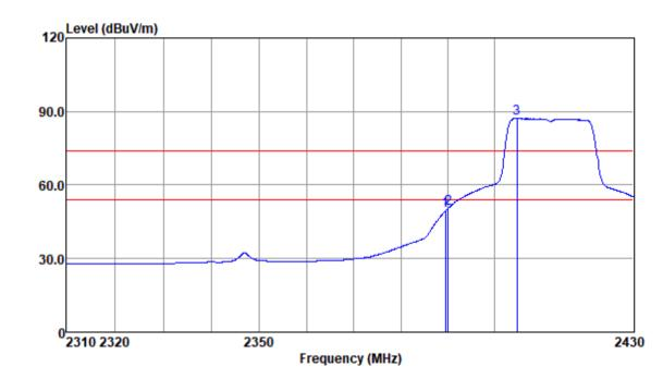
Mode:a; Polarization:Vertical; Modulation:n; bandwidth:20MHz; Channel:Low
