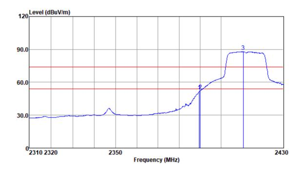
Mode:a; Polarization:Horizontal; Modulation:n; bandwidth:20MHz; Channel:Low
