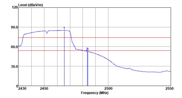
Mode:a; Polarization:Horizontal; Modulation:n; bandwidth:40MHz; Channel:High
