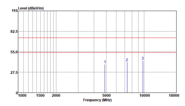
Mode:a; Polarization:Vertical; Modulation:b; bandwidth:20MHz; Channel:middle
