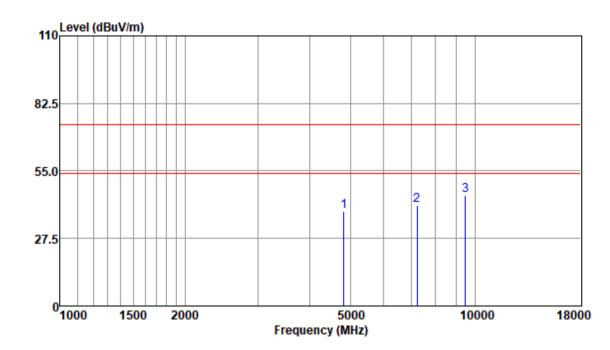
Mode:a; Polarization:Vertical; Modulation:b; bandwidth:20MHz; Channel:Low
