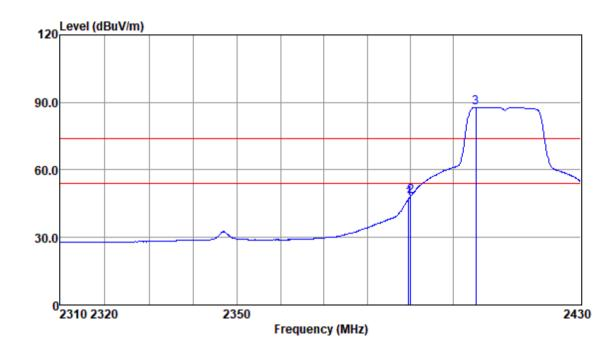
Mode:a; Polarization:Vertical; Modulation:g; bandwidth:20MHz; Channel:Low
