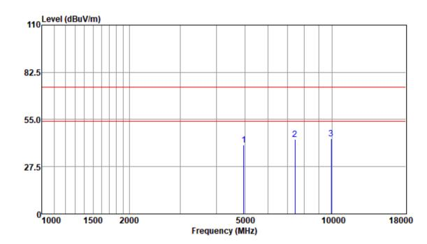
Mode:a; Polarization:Horizontal; Modulation:n; bandwidth:20MHz; Channel:High
