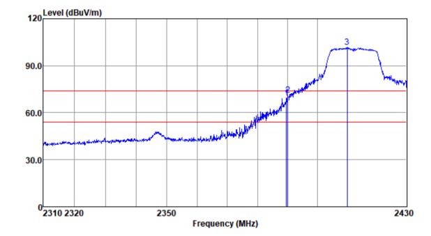
Mode:a; Polarization:Horizontal; Modulation:g; bandwidth:20MHz; Channel:Low
