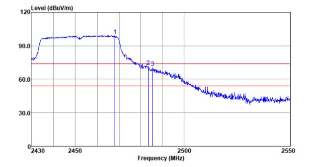
Mode:a; Polarization:Horizontal; Modulation:n; bandwidth:40MHz; Channel:High
