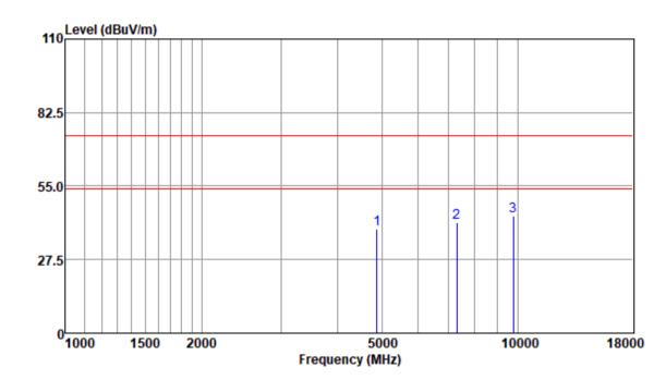
Mode:a; Polarization:Vertical; Modulation:n; bandwidth:40MHz; Channel:middle
