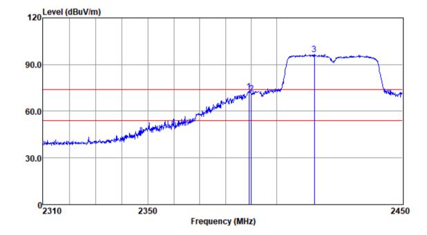
Mode:a; Polarization:Vertical; Modulation:n; bandwidth:40MHz; Channel:Low
