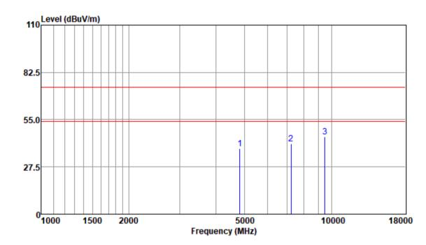
Mode:a; Polarization:Vertical; Modulation:g; bandwidth:20MHz; Channel:Low
