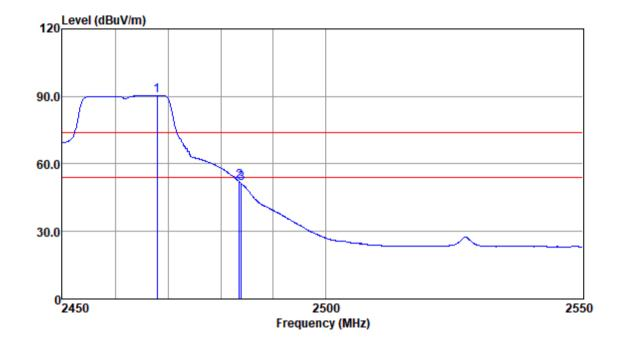
Mode:a; Polarization:Horizontal; Modulation:g; bandwidth:20MHz; Channel:High
