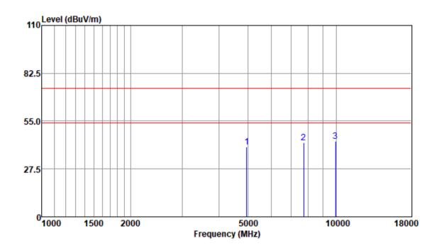
Mode:a; Polarization:Vertical; Modulation:b; bandwidth:20MHz; Channel:High
