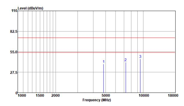
Mode:a; Polarization:Vertical; Modulation:n; bandwidth:20MHz; Channel:Low
