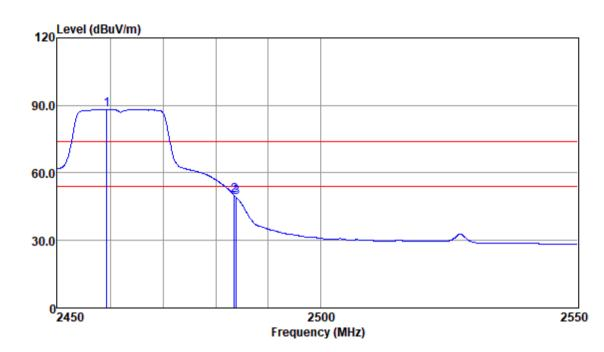
Mode:a; Polarization:Vertical; Modulation:g; bandwidth:20MHz; Channel:High
