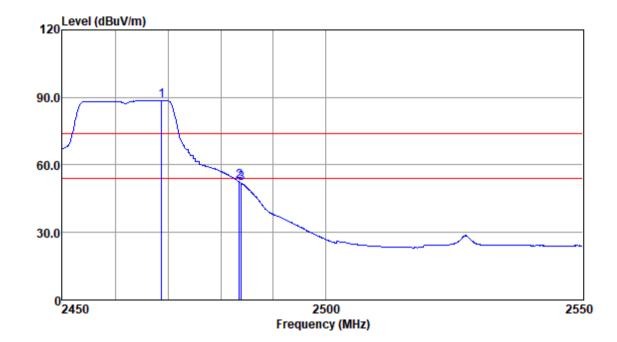
Mode:a; Polarization:Horizontal; Modulation:n; bandwidth:20MHz; Channel:High
