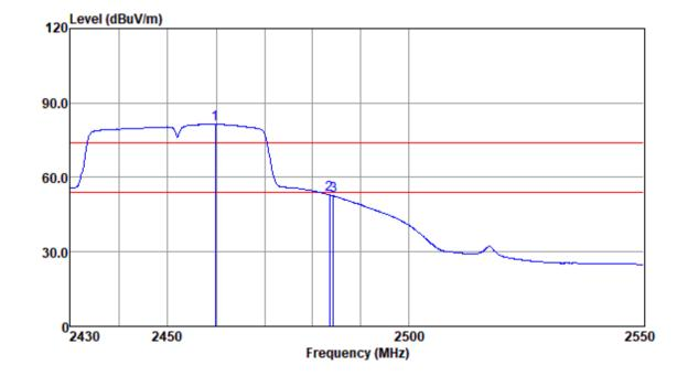
Mode:a; Polarization:Vertical; Modulation:n; bandwidth:40MHz; Channel:High
