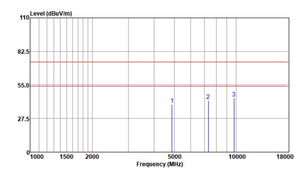
Mode:a; Polarization:Vertical; Modulation:n; bandwidth:20MHz; Channel:middle
