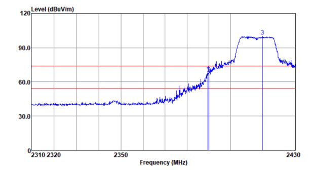
Mode:a; Polarization:Vertical; Modulation:g; bandwidth:20MHz; Channel:Low
