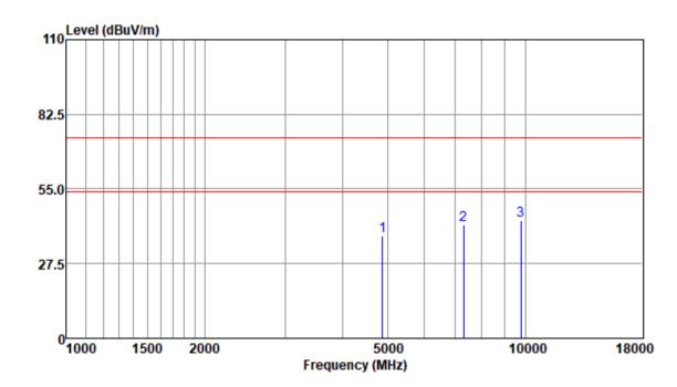
Mode:a; Polarization:Horizontal; Modulation:n; bandwidth:40MHz; Channel:middle
