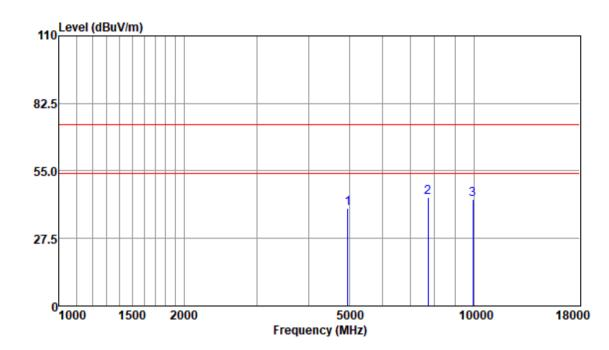
Mode:a; Polarization:Vertical; Modulation:g; bandwidth:20MHz; Channel:High
