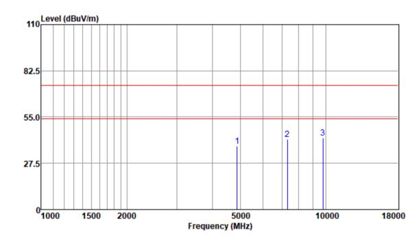
Mode:a; Polarization:Horizontal; Modulation:n; bandwidth:20MHz; Channel:middle
