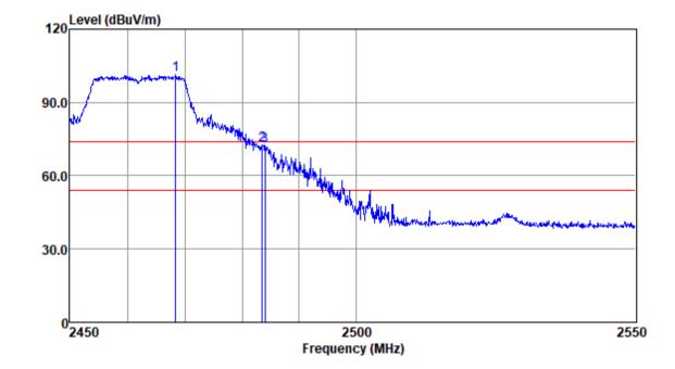
Mode:a; Polarization:Horizontal; Modulation:g; bandwidth:20MHz; Channel:High
