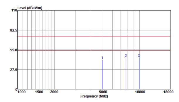
Mode:a; Polarization:Horizontal; Modulation:b; bandwidth:20MHz; Channel:High
