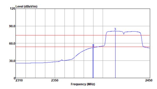
Mode:a; Polarization:Vertical; Modulation:n; bandwidth:40MHz; Channel:Low
