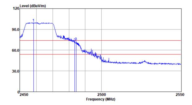
Mode:a; Polarization:Vertical; Modulation:n; bandwidth:20MHz; Channel:High
