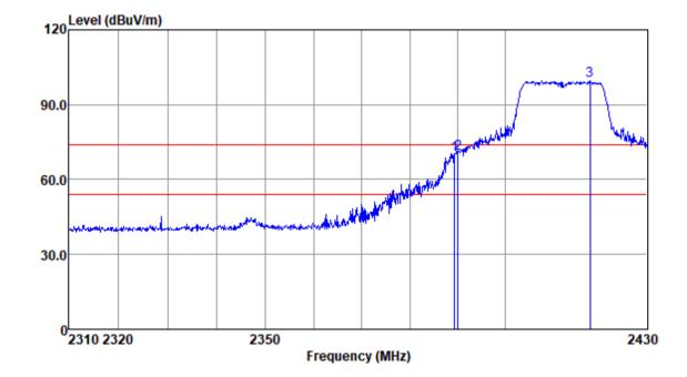
Mode:a; Polarization:Vertical; Modulation:n; bandwidth:20MHz; Channel:Low
