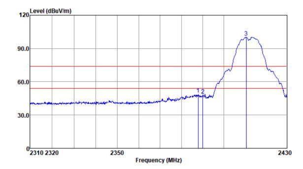
Mode:a; Polarization:Vertical; Modulation:b; bandwidth:20MHz; Channel:Low
