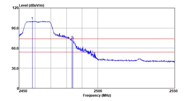
Mode:a; Polarization:Vertical; Modulation:g; bandwidth:20MHz; Channel:High
