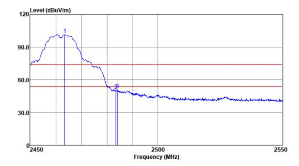
Mode:a; Polarization:Horizontal; Modulation:b; bandwidth:20MHz; Channel:High
