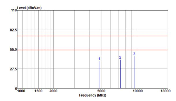
Mode:a; Polarization:Vertical; Modulation:n; bandwidth:40MHz; Channel:Low
