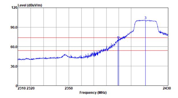
Mode:a; Polarization:Horizontal; Modulation:n; bandwidth:20MHz; Channel:Low
