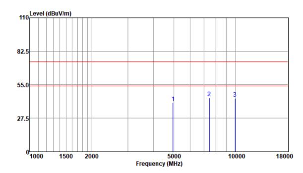
Mode:a; Polarization:Horizontal; Modulation:n; bandwidth:40MHz; Channel:High
