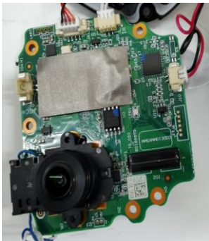
Before change: Integral Antenna, Antenna Gain: 2.3dBi,
