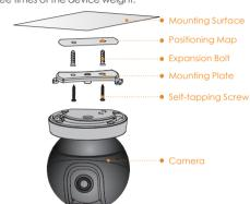
Step1 Drill screw holes on the mounting surface as the mounting plate shows, and then put in the expansion bolts.
