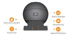
Note: Press the Reset/WPS button to enable WPS. Press and hold the Reset/WPS button for 10 s to reset the camera.
