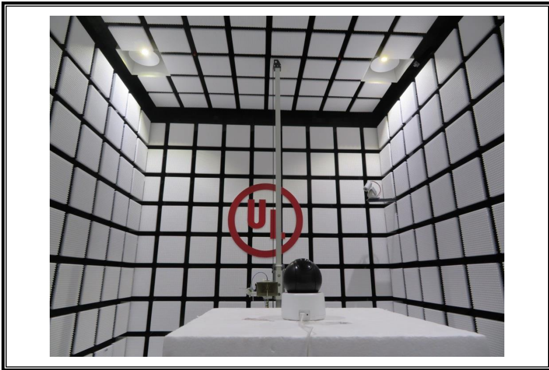
POWERLINE CONDUCTED EMISSIONS MEASUREMENT SETUP
