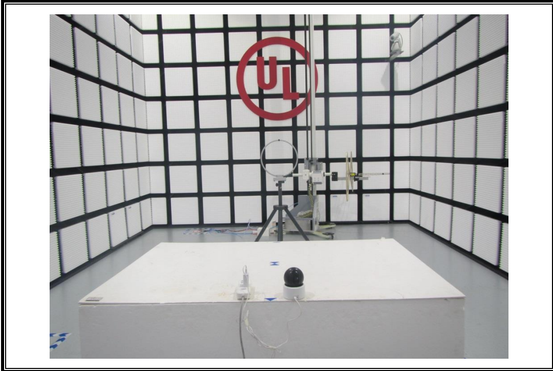
RADIATED RF MEASUREMENT SETUP (30MHz ~ 1 GHz)
