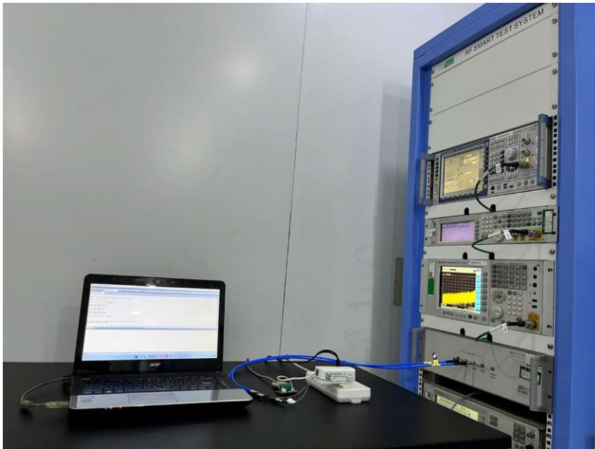
RF conducted setup
