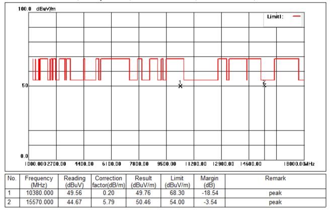
Test Mode: 01; Polarity: Vertical; Modulation:802.11ac; Bandwidth:40MHz; Channel:Low
