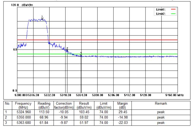
Test Mode: 02; Polarity: Horizontal; Modulation:802.11ac; Bandwidth:20MHz; Channel:High
