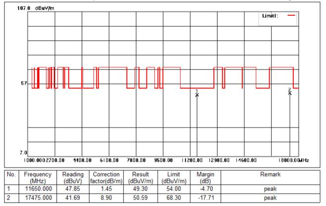
Test Mode: 04; Polarity: Horizontal; Modulation:802.11ac; Bandwidth:20MHz; Channel:High
