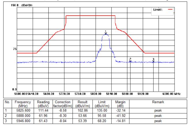
Test Mode: 04; Polarity: Vertical; Modulation:802.11ac; Bandwidth:20MHz; Channel:High
