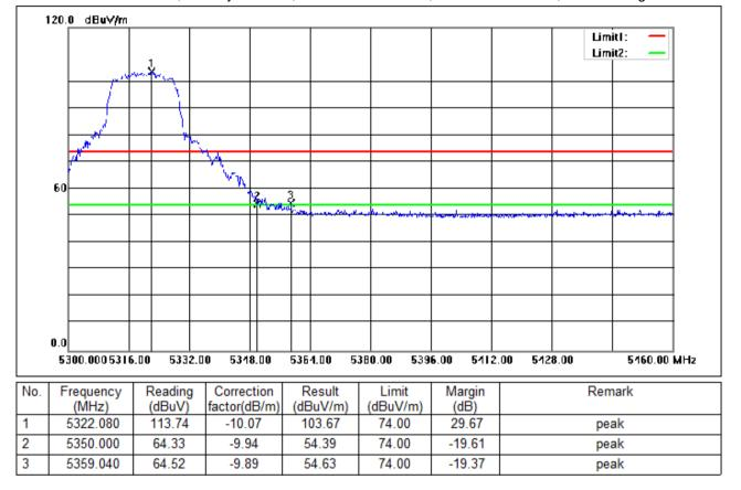
Test Mode: 02; Polarity: Vertical; Modulation:802.11n; Bandwidth:20MHz; Channel:High
