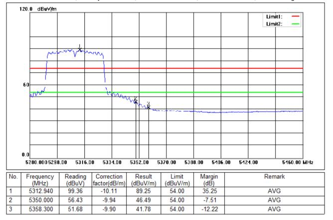
Test Mode: 02; Polarity: Horizontal; Modulation:802.11n; Bandwidth:40MHz; Channel:High
