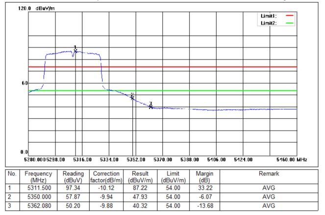
Test Mode: 02; Polarity: Vertical; Modulation:802.11ac; Bandwidth:40MHz; Channel:High
