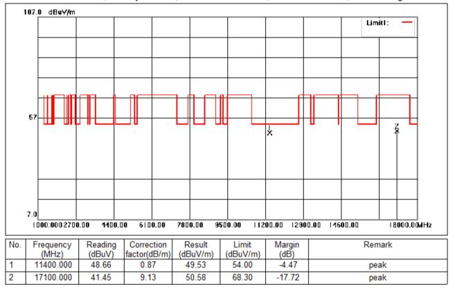
Test Mode: 03; Polarity: Vertical; Modulation:802.11ac; Bandwidth:20MHz; Channel:High
