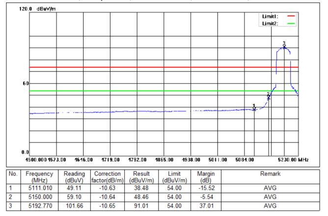
Test Mode: 01; Polarity: Vertical; Modulation:802.11n; Bandwidth:40MHz; Channel:Low
