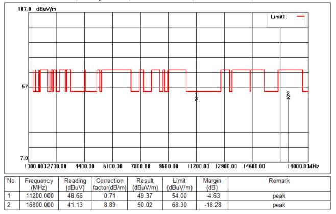
Test Mode: 03; Polarity: Vertical; Modulation:802.11n; Bandwidth:20MHz; Channel:middle
