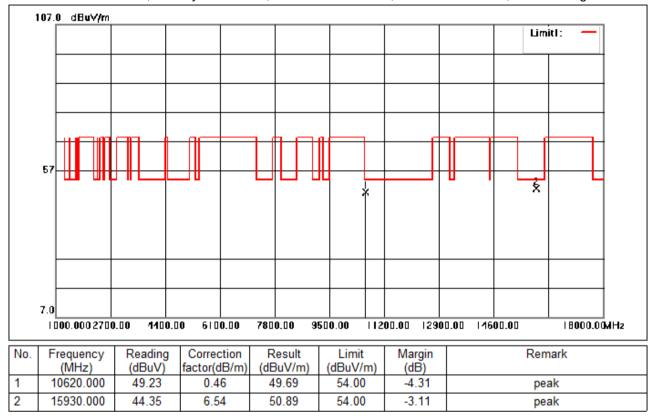
Test Mode: 02; Polarity: Horizontal; Modulation:802.11n; Bandwidth:40MHz; Channel:High
