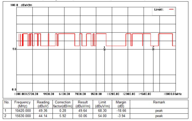
Test Mode: 01; Polarity: Vertical; Modulation:802.11ac; Bandwidth:80MHz; Channel:middle
