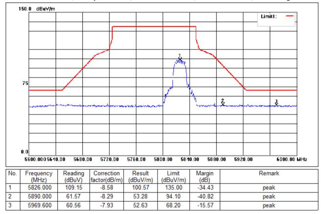
Test Mode: 04; Polarity: Horizontal; Modulation:802.11ac; Bandwidth:20MHz; Channel:High
