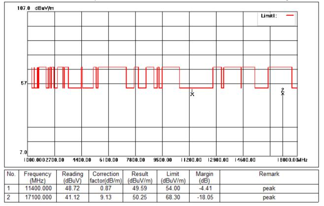
Test Mode: 03; Polarity: Horizontal; Modulation:802.11a; Bandwidth:20MHz; Channel:High
