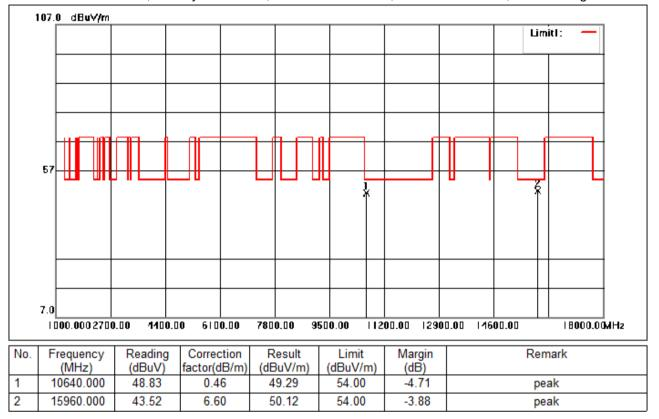
Test Mode: 02; Polarity: Horizontal; Modulation:802.11a; Bandwidth:20MHz; Channel:High
