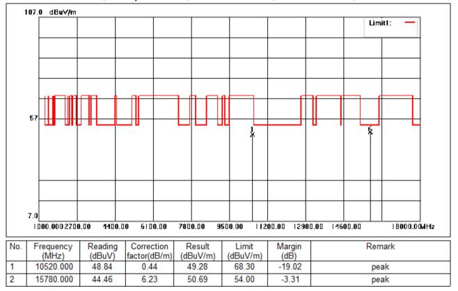
Test Mode: 02; Polarity: Horizontal; Modulation:802.11n; Bandwidth:20MHz; Channel:Low
