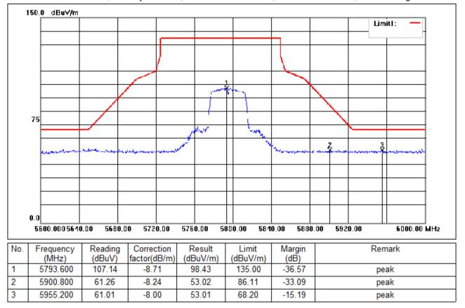
Test Mode: 04; Polarity: Vertical; Modulation:802.11ac; Bandwidth:40MHz; Channel:High
