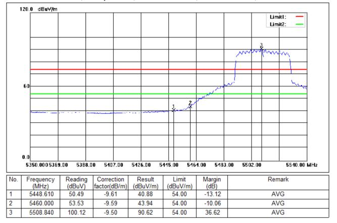
Test Mode: 03; Polarity: Vertical; Modulation:802.11n; Bandwidth:40MHz; Channel:Low
