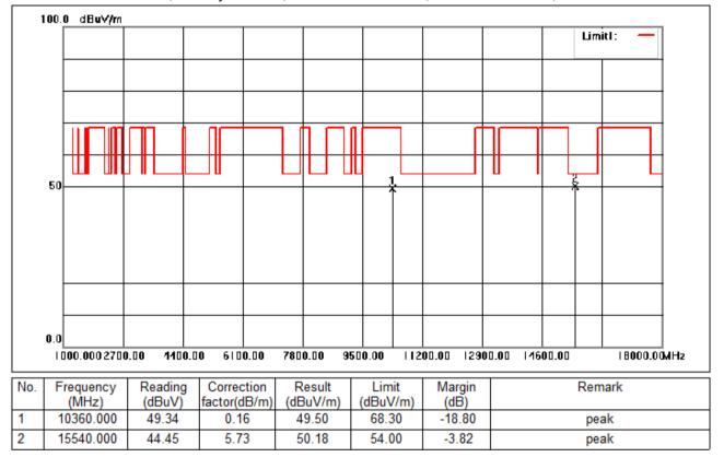
Test Mode: 01; Polarity: Vertical; Modulation:802.11ac; Bandwidth:20MHz; Channel:Low
