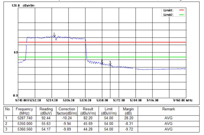
Test Mode: 02; Polarity: Horizontal; Modulation:802.11ac; Bandwidth:80MHz; Channel:High
