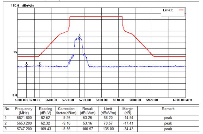
Test Mode: 04; Polarity: Horizontal; Modulation:802.11ac; Bandwidth:20MHz; Channel:Low
