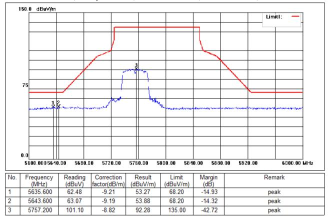
Test Mode: 04; Polarity: Horizontal; Modulation:802.11ac; Bandwidth:40MHz; Channel:Low
