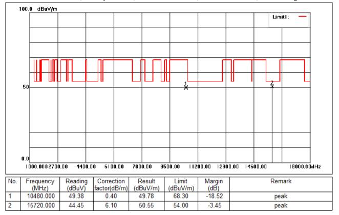
Test Mode: 01; Polarity: Vertical; Modulation:802.11n; Bandwidth:20MHz; Channel:High
