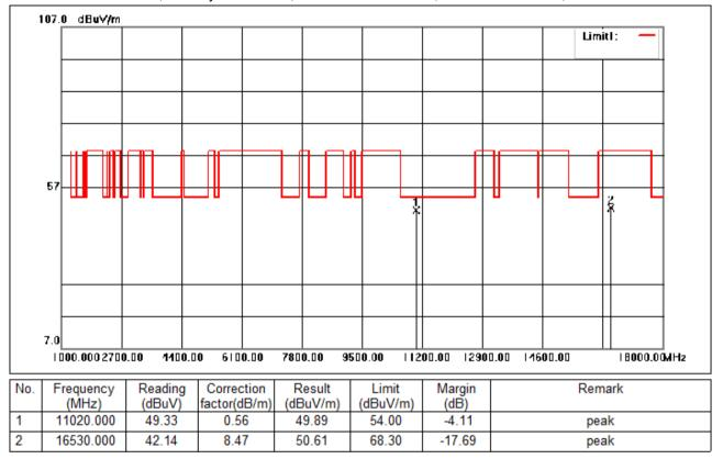
Test Mode: 03; Polarity: Horizontal; Modulation:802.11ac; Bandwidth:40MHz; Channel:Low
