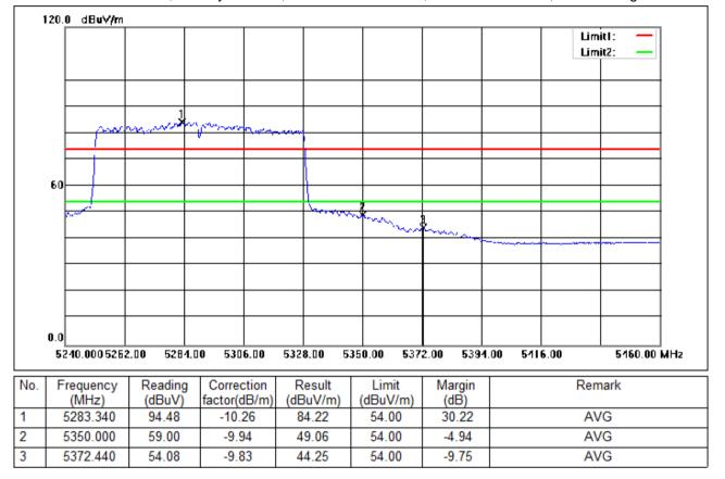
Test Mode: 02; Polarity: Vertical; Modulation:802.11ac; Bandwidth:80MHz; Channel:High
