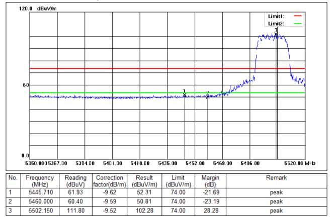
Test Mode: 03; Polarity: Horizontal; Modulation:802.11ac; Bandwidth:20MHz; Channel:Low
