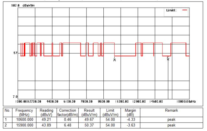
Test Mode: 02; Polarity: Horizontal; Modulation:802.11n; Bandwidth:20MHz; Channel:middle
