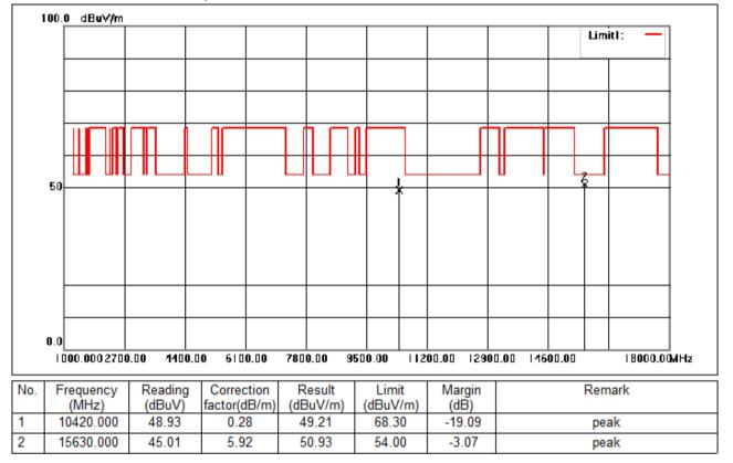
Test Mode: 01; Polarity: Horizontal; Modulation:802.11ac; Bandwidth:80MHz; Channel:middle
