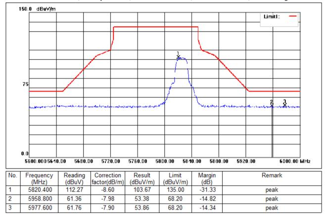
Test Mode: 04; Polarity: Vertical; Modulation:802.11a; Bandwidth:20MHz; Channel:High
