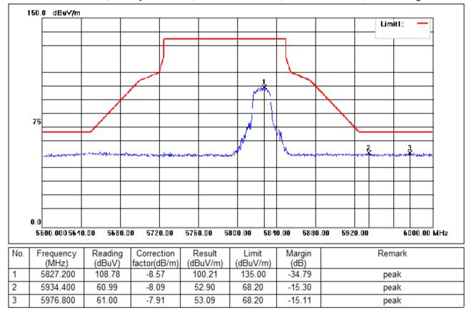
Test Mode: 04; Polarity: Horizontal; Modulation:802.11n; Bandwidth:20MHz; Channel:High
