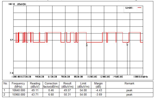
Test Mode: 02; Polarity: Vertical; Modulation:802.11a; Bandwidth:20MHz; Channel:High
