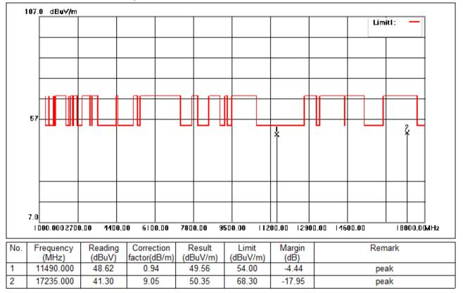
Test Mode: 04; Polarity: Horizontal; Modulation:802.11ac; Bandwidth:20MHz; Channel:Low
