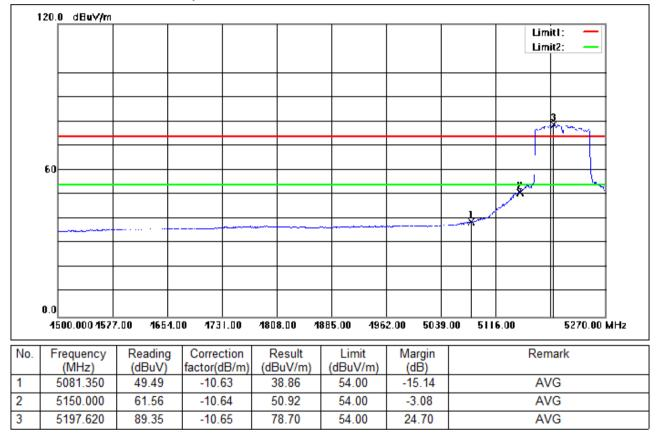
Test Mode: 01; Polarity: Horizontal; Modulation:802.11ac; Bandwidth:80MHz; Channel:Low
