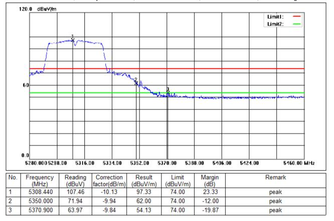
Test Mode: 02; Polarity: Horizontal; Modulation:802.11ac; Bandwidth:40MHz; Channel:High
