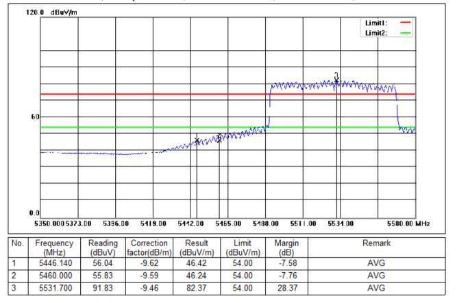
Test Mode: 03; Polarity: Horizontal; Modulation:802.11ac; Bandwidth:80MHz; Channel:Low
