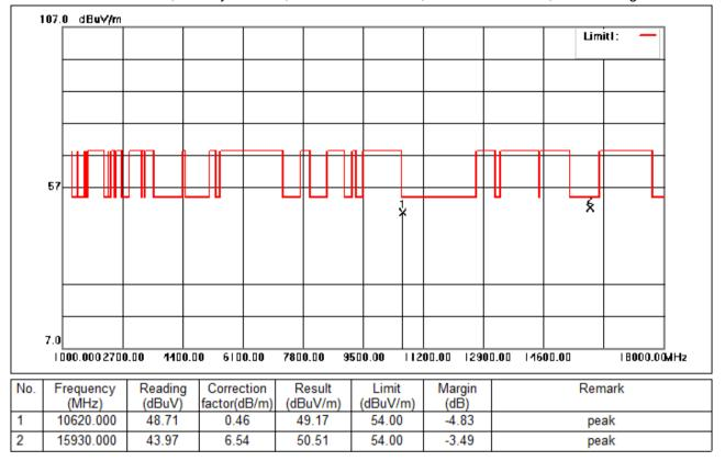
Test Mode: 02; Polarity: Vertical; Modulation:802.11n; Bandwidth:40MHz; Channel:High
