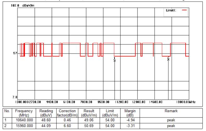
Test Mode: 02; Polarity: Horizontal; Modulation:802.11ac; Bandwidth:20MHz; Channel:High
