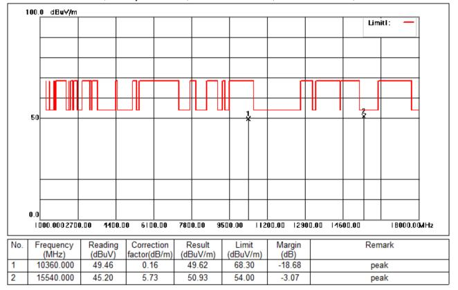
Test Mode: 01; Polarity: Horizontal; Modulation:802.11n; Bandwidth:20MHz; Channel:Low
