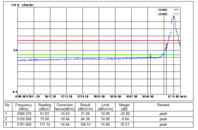
Test Mode: 01; Polarity: Vertical; Modulation:802.11ac; Bandwidth:20MHz; Channel:Low
