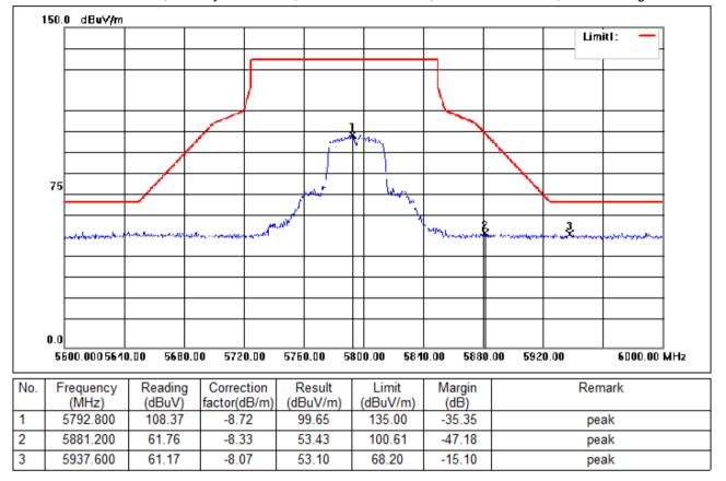
Test Mode: 04; Polarity: Horizontal; Modulation:802.11n; Bandwidth:40MHz; Channel:High
