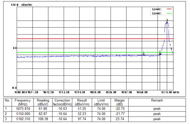
Test Mode: 01; Polarity: Horizontal; Modulation:802.11a; Bandwidth:20MHz; Channel:Low
