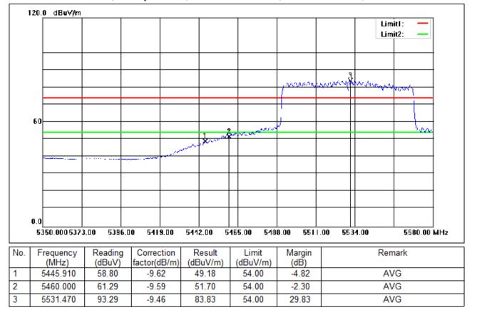
Test Mode: 03; Polarity: Vertical; Modulation:802.11ac; Bandwidth:80MHz; Channel:Low
