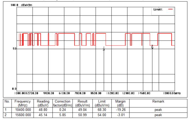
Test Mode: 01; Polarity: Vertical; Modulation:802.11n; Bandwidth:20MHz; Channel:middle
