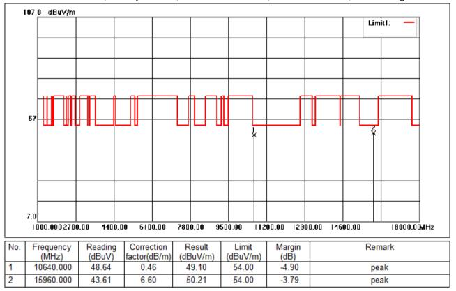
Test Mode: 02; Polarity: Vertical; Modulation:802.11ac; Bandwidth:20MHz; Channel:High
