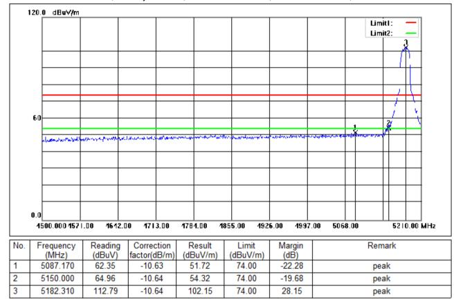
Test Mode: 01; Polarity: Vertical; Modulation:802.11a; Bandwidth:20MHz; Channel:Low
