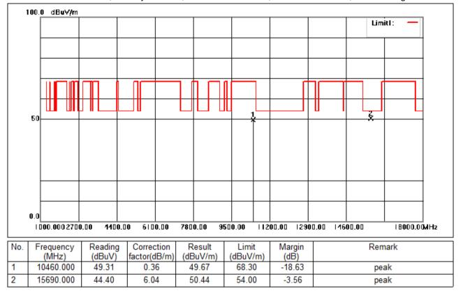
Test Mode: 01; Polarity: Vertical; Modulation:802.11n; Bandwidth:40MHz; Channel:High
