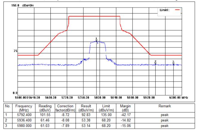
Test Mode: 04; Polarity: Horizontal; Modulation:802.11ac; Bandwidth:40MHz; Channel:High
