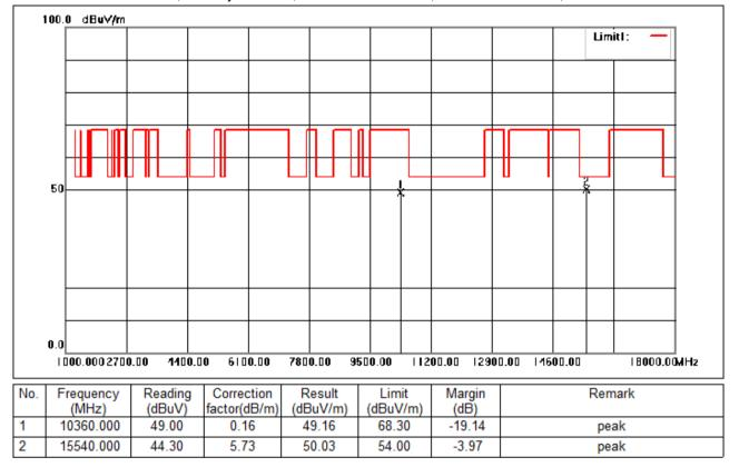
Test Mode: 01; Polarity: Vertical; Modulation:802.11a; Bandwidth:20MHz; Channel:Low
