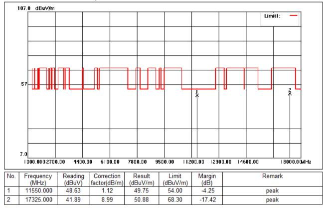
Test Mode: 04; Polarity: Vertical; Modulation:802.11ac; Bandwidth:80MHz; Channel:middle
