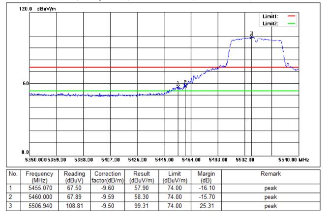
Test Mode: 03; Polarity: Vertical; Modulation:802.11ac; Bandwidth:40MHz; Channel:Low
