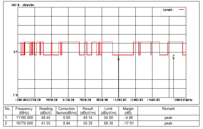
Test Mode: 03; Polarity: Horizontal; Modulation:802.11ac; Bandwidth:40MHz; Channel:middle
