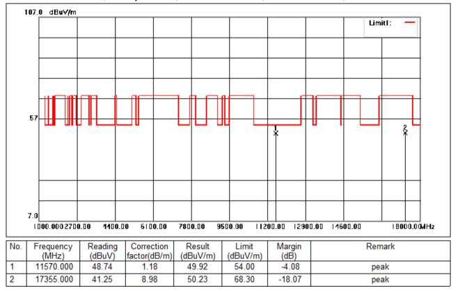
Test Mode: 04; Polarity: Vertical; Modulation:802.11n; Bandwidth:20MHz; Channel:middle
