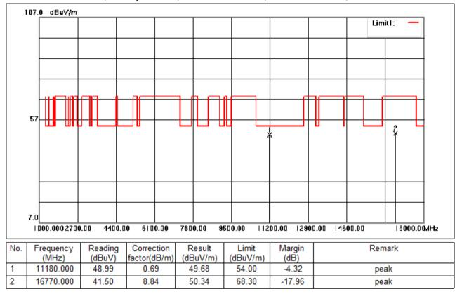
Test Mode: 03; Polarity: Vertical; Modulation:802.11n; Bandwidth:40MHz; Channel:middle
