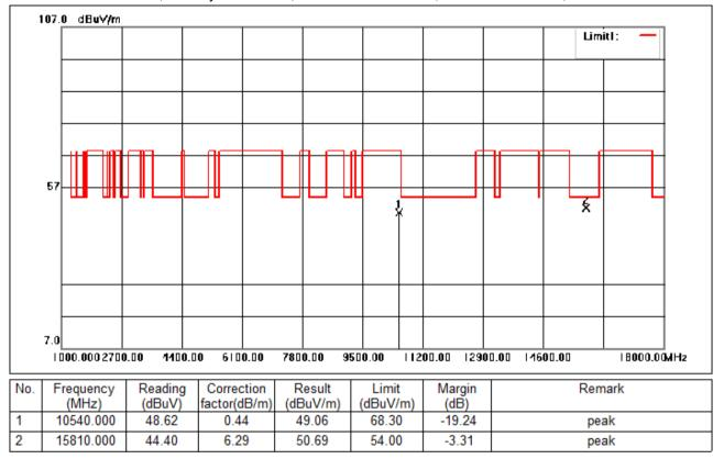
Test Mode: 02; Polarity: Horizontal; Modulation:802.11ac; Bandwidth:40MHz; Channel:Low
