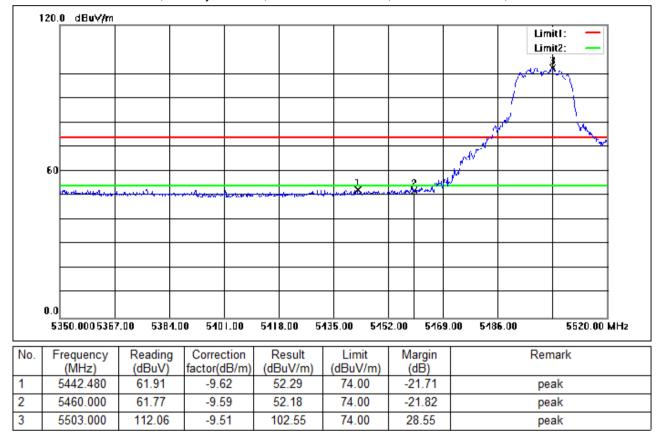
Test Mode: 03; Polarity: Vertical; Modulation:802.11n; Bandwidth:20MHz; Channel:Low
