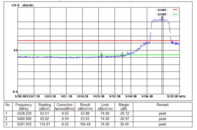
Test Mode: 03; Polarity: Vertical; Modulation:802.11ac; Bandwidth:20MHz; Channel:Low
