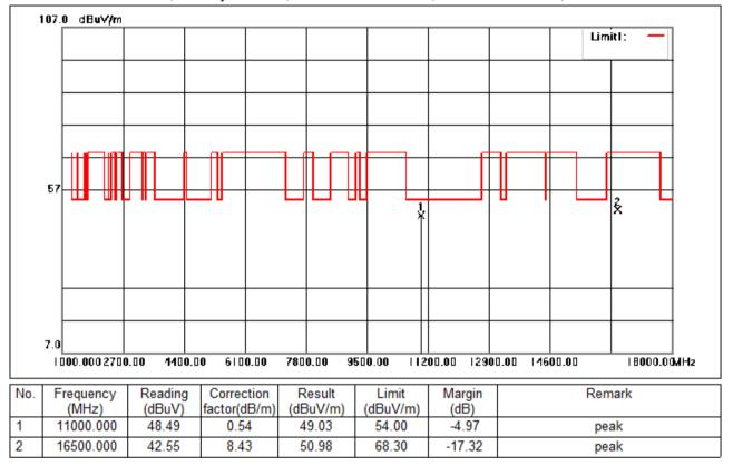
Test Mode: 03; Polarity: Vertical; Modulation:802.11ac; Bandwidth:20MHz; Channel:Low
