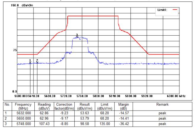
Test Mode: 04; Polarity: Vertical; Modulation:802.11n; Bandwidth:40MHz; Channel:Low
