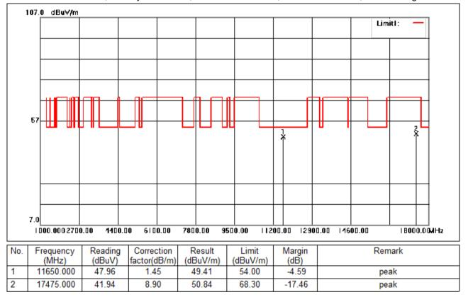
Test Mode: 04; Polarity: Horizontal; Modulation:802.11n; Bandwidth:20MHz; Channel:High
