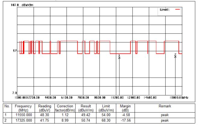
Test Mode: 04; Polarity: Horizontal; Modulation:802.11ac; Bandwidth:80MHz; Channel:middle
