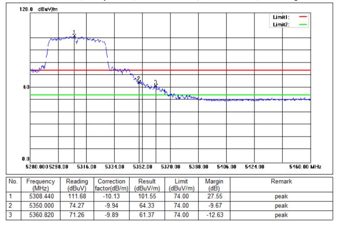
Test Mode: 02; Polarity: Vertical; Modulation:802.11n; Bandwidth:40MHz; Channel:High
