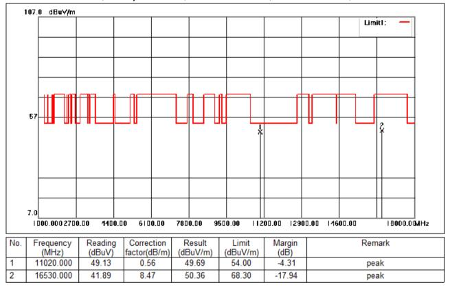
Test Mode: 03; Polarity: Horizontal; Modulation:802.11n; Bandwidth:40MHz; Channel:Low
