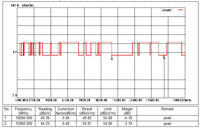
Test Mode: 02; Polarity: Vertical; Modulation:802.11a; Bandwidth:20MHz; Channel:middle
