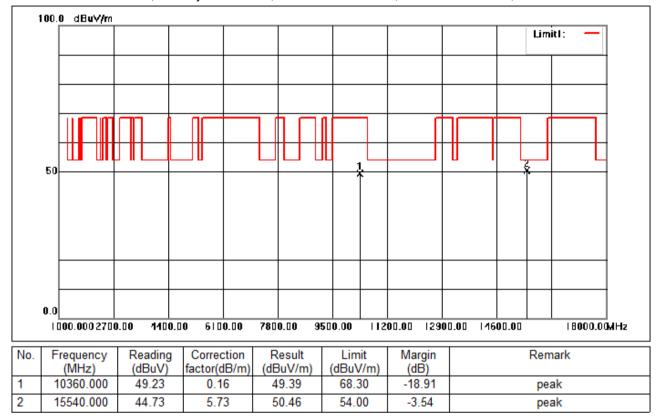
Test Mode: 01; Polarity: Horizontal; Modulation:802.11a; Bandwidth:20MHz; Channel:Low
