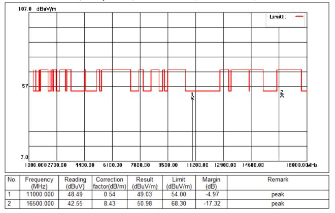
Test Mode: 03; Polarity: Vertical; Modulation:802.11n; Bandwidth:20MHz; Channel:Low
