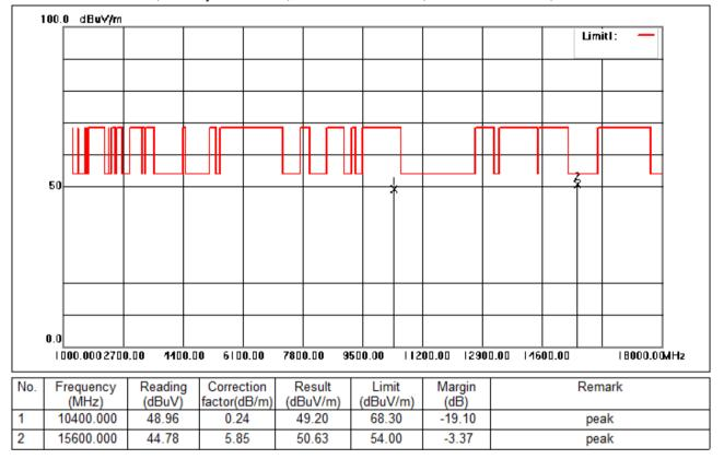
Test Mode: 01; Polarity: Horizontal; Modulation:802.11a; Bandwidth:20MHz; Channel:middle
