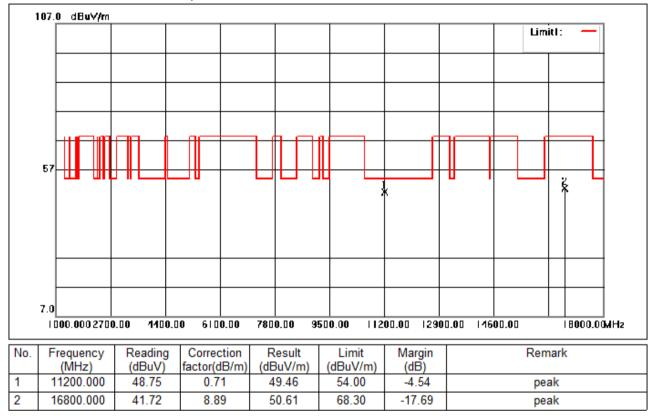
Test Mode: 03; Polarity: Vertical; Modulation:802.11ac; Bandwidth:20MHz; Channel:middle
