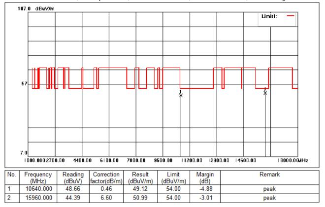
Test Mode: 02; Polarity: Vertical; Modulation:802.11n; Bandwidth:20MHz; Channel:High
