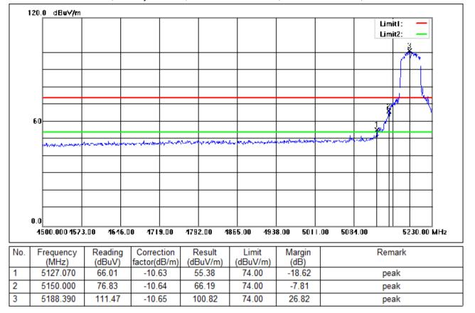
Test Mode: 01; Polarity: Vertical; Modulation:802.11ac; Bandwidth:40MHz; Channel:Low
