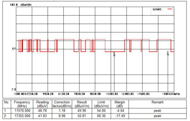
Test Mode: 04; Polarity: Horizontal; Modulation:802.11n; Bandwidth:20MHz; Channel:middle
