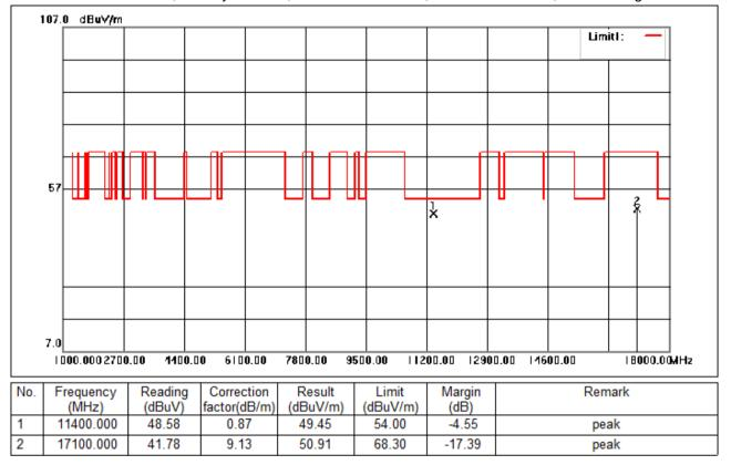
Test Mode: 03; Polarity: Vertical; Modulation:802.11a; Bandwidth:20MHz; Channel:High
