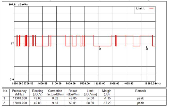
Test Mode: 03; Polarity: Vertical; Modulation:802.11ac; Bandwidth:40MHz; Channel:High
