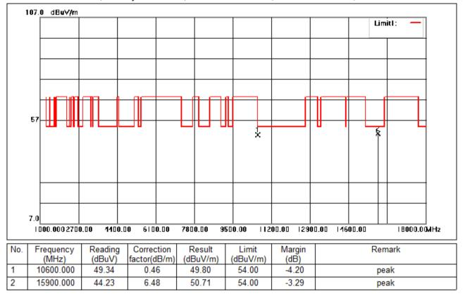
Test Mode: 02; Polarity: Horizontal; Modulation:802.11a; Bandwidth:20MHz; Channel:middle
