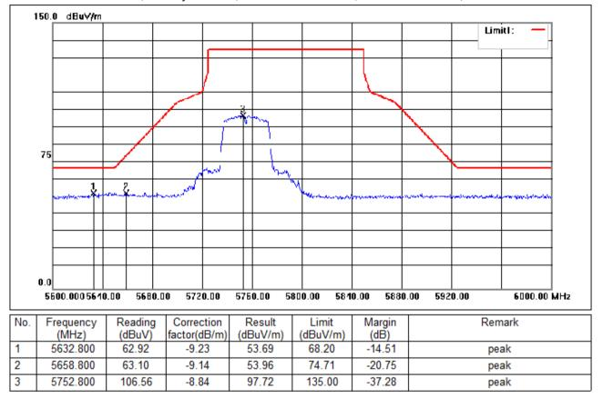
Test Mode: 04; Polarity: Vertical; Modulation:802.11ac; Bandwidth:40MHz; Channel:Low
