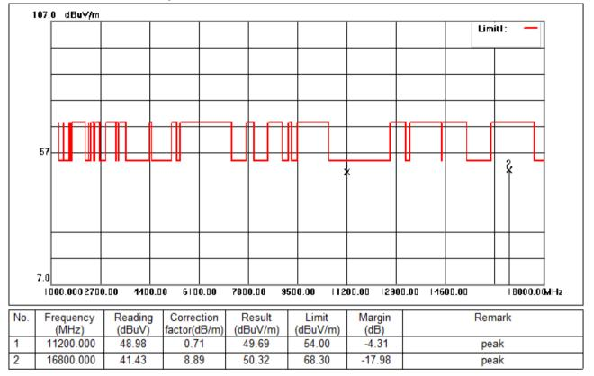
Test Mode: 03; Polarity: Horizontal; Modulation:802.11a; Bandwidth:20MHz; Channel:middle
