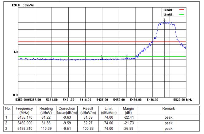
Test Mode: 03; Polarity: Horizontal; Modulation:802.11n; Bandwidth:20MHz; Channel:Low
