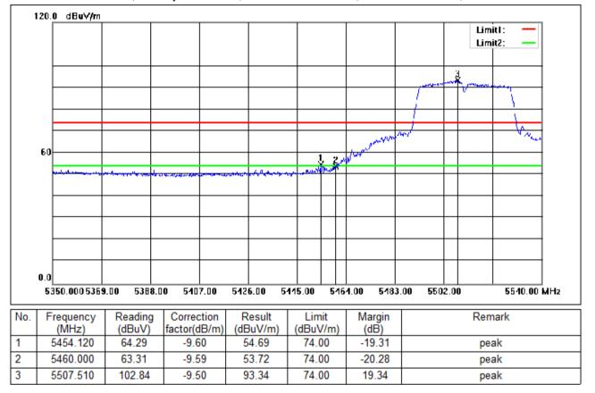
Test Mode: 03; Polarity: Horizontal; Modulation:802.11ac; Bandwidth:40MHz; Channel:Low
