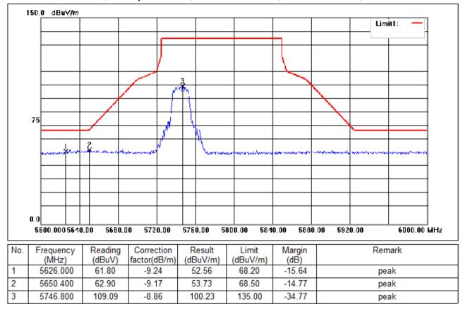
Test Mode: 04; Polarity: Horizontal; Modulation:802.11n; Bandwidth:20MHz; Channel:Low
