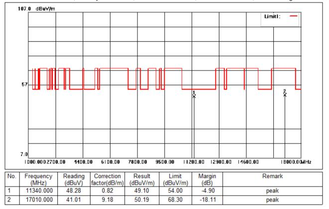
Test Mode: 03; Polarity: Horizontal; Modulation:802.11n; Bandwidth:40MHz; Channel:High
