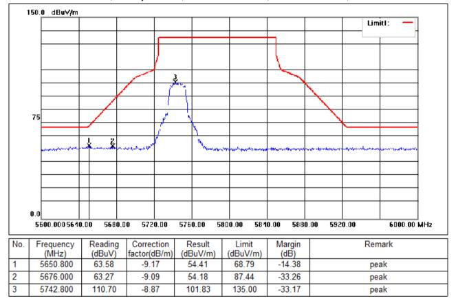
Test Mode: 04; Polarity: Vertical; Modulation:802.11n; Bandwidth:20MHz; Channel:Low
