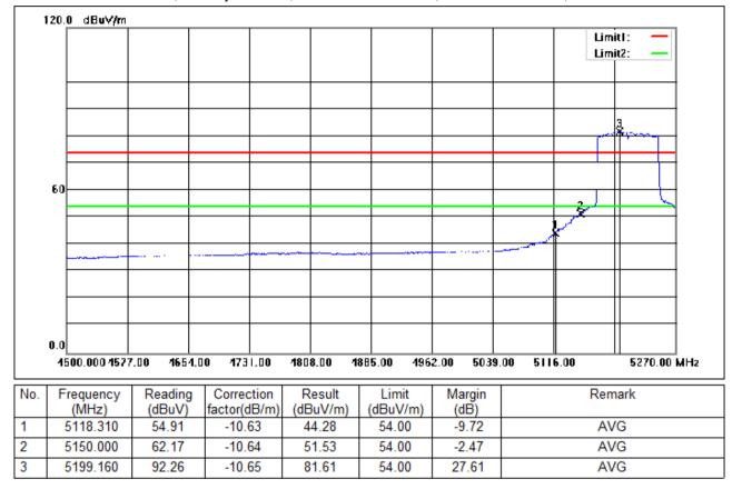
Test Mode: 01; Polarity: Vertical; Modulation:802.11ac; Bandwidth:80MHz; Channel:Low
