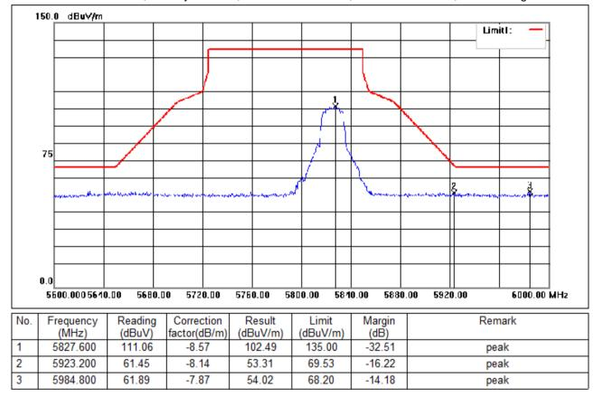
Test Mode: 04; Polarity: Vertical; Modulation:802.11n; Bandwidth:20MHz; Channel:High
