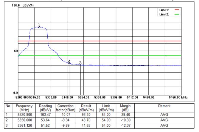
Test Mode: 02; Polarity: Vertical; Modulation:802.11a; Bandwidth:20MHz; Channel:High
