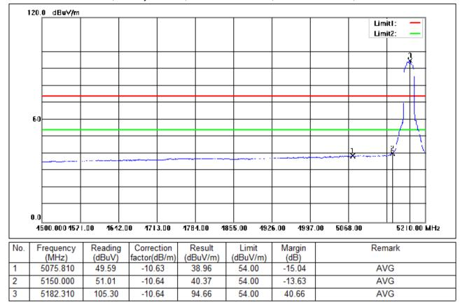
Test Mode: 01; Polarity: Vertical; Modulation:802.11n; Bandwidth:20MHz; Channel:Low
