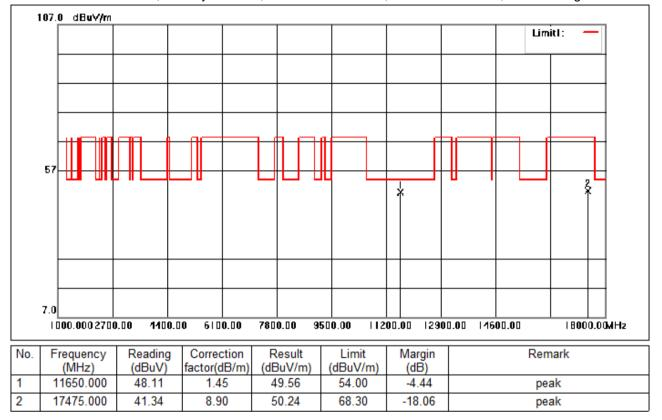
Test Mode: 04; Polarity: Vertical; Modulation:802.11a; Bandwidth:20MHz; Channel:High
