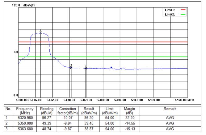
Test Mode: 02; Polarity: Horizontal; Modulation:802.11a; Bandwidth:20MHz; Channel:High
