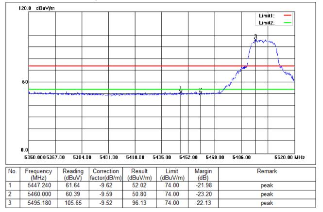
Test Mode: 03; Polarity: Horizontal; Modulation:802.11a; Bandwidth:20MHz; Channel:Low
