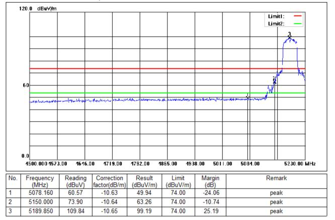
Test Mode: 01; Polarity: Horizontal; Modulation:802.11n; Bandwidth:40MHz; Channel:Low
