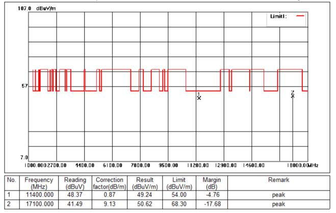
Test Mode: 03; Polarity: Horizontal; Modulation:802.11ac; Bandwidth:20MHz; Channel:High
