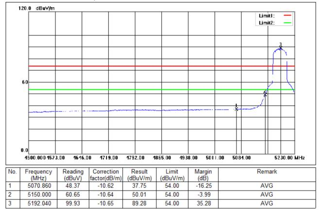
Test Mode: 01; Polarity: Horizontal; Modulation:802.11ac; Bandwidth:40MHz; Channel:Low
