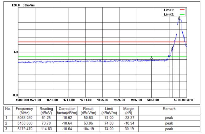
Test Mode: 01; Polarity: Horizontal; Modulation:802.11ac; Bandwidth:20MHz; Channel:Low
