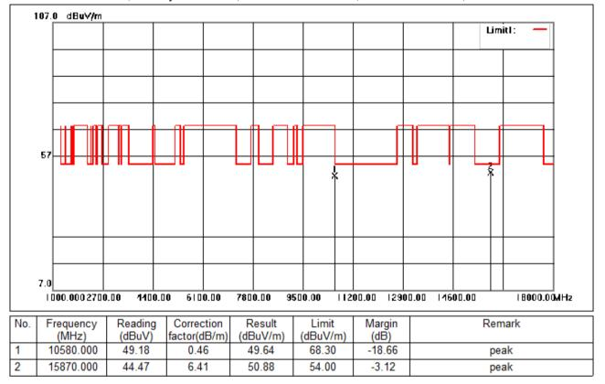
Test Mode: 02; Polarity: Horizontal; Modulation:802.11ac; Bandwidth:80MHz; Channel:middle
