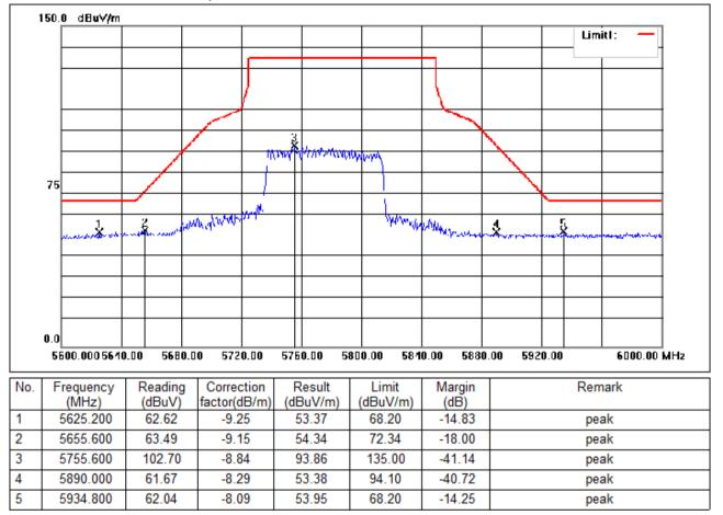
Test Mode: 04; Polarity: Horizontal; Modulation:802.11ac; Bandwidth:80MHz; Channel:Low
