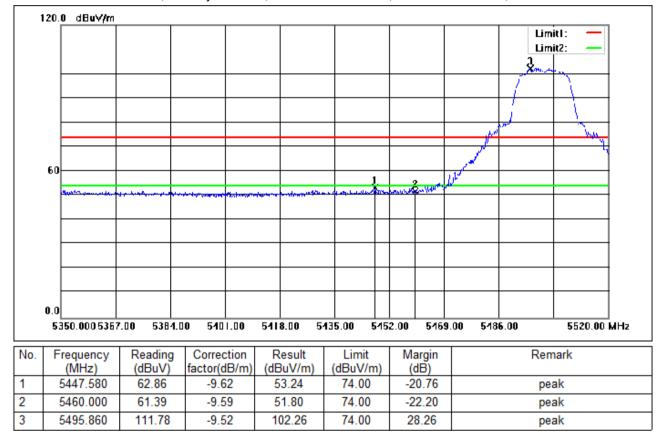
Test Mode: 03; Polarity: Vertical; Modulation:802.11a; Bandwidth:20MHz; Channel:Low
