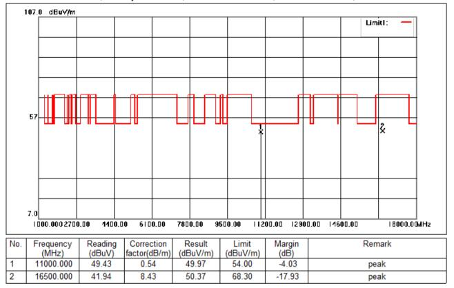
Test Mode: 03; Polarity: Horizontal; Modulation:802.11ac; Bandwidth:20MHz; Channel:Low
