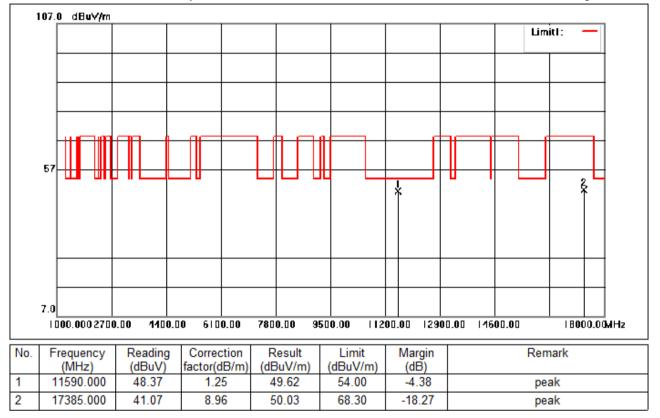
Test Mode: 04; Polarity: Horizontal; Modulation:802.11ac; Bandwidth:40MHz; Channel:High
