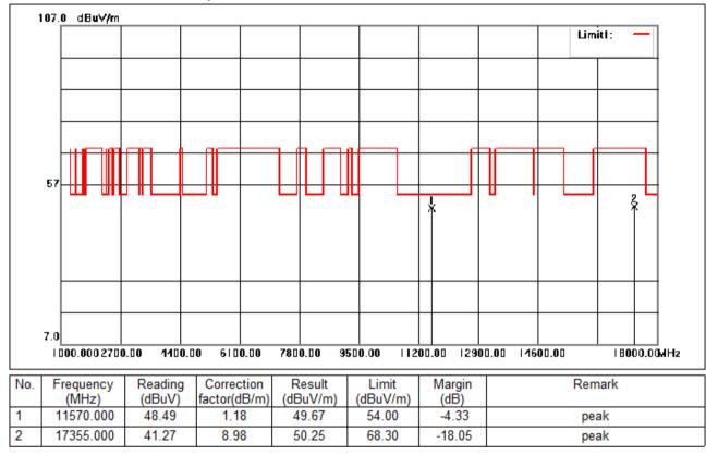
Test Mode: 04; Polarity: Vertical; Modulation:802.11ac; Bandwidth:20MHz; Channel:middle
