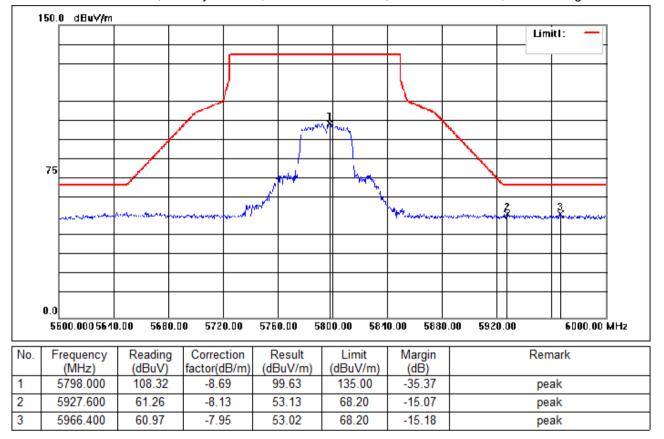
Test Mode: 04; Polarity: Vertical; Modulation:802.11n; Bandwidth:40MHz; Channel:High
