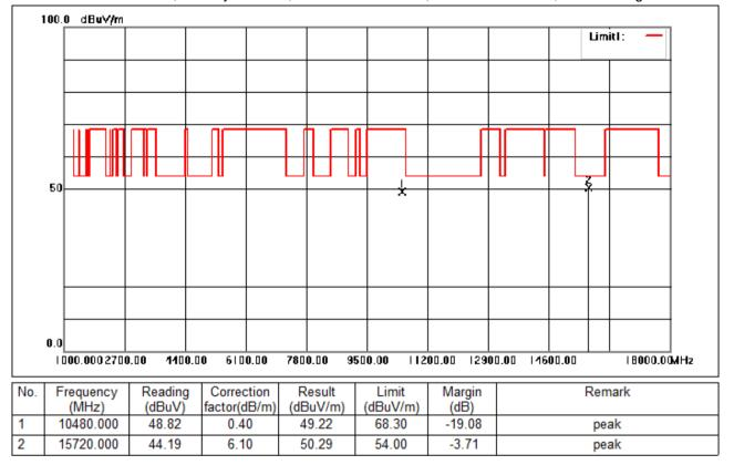
Test Mode: 01; Polarity: Vertical; Modulation:802.11a; Bandwidth:20MHz; Channel:High
