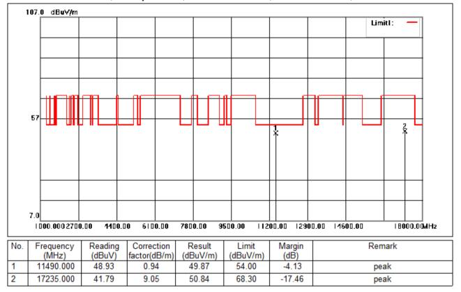
Test Mode: 04; Polarity: Vertical; Modulation:802.11n; Bandwidth:20MHz; Channel:Low
