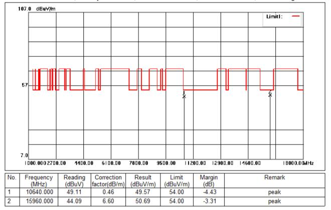
Test Mode: 02; Polarity: Horizontal; Modulation:802.11n; Bandwidth:20MHz; Channel:High
