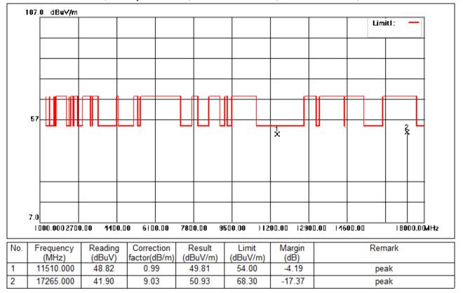
Test Mode: 04; Polarity: Horizontal; Modulation:802.11n; Bandwidth:40MHz; Channel:Low
