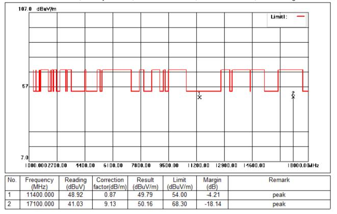
Test Mode: 03; Polarity: Vertical; Modulation:802.11n; Bandwidth:20MHz; Channel:High
