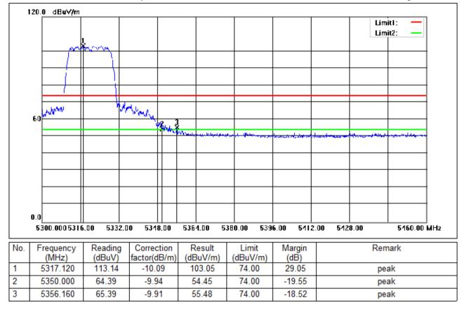
Test Mode: 02; Polarity: Vertical; Modulation:802.11ac; Bandwidth:20MHz; Channel:High
