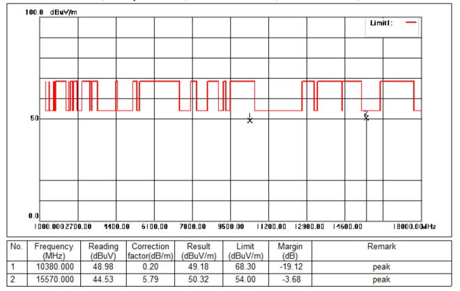
Test Mode: 01; Polarity: Horizontal; Modulation:802.11ac; Bandwidth:40MHz; Channel:Low
