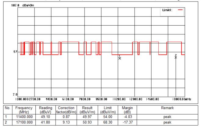
Test Mode: 03; Polarity: Horizontal; Modulation:802.11n; Bandwidth:20MHz; Channel:High
