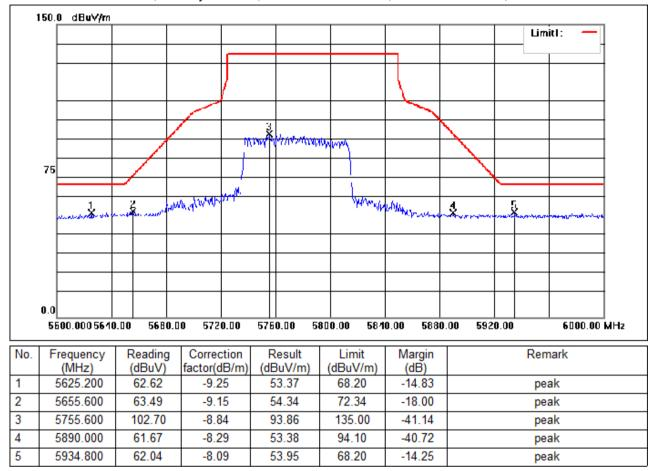
Test Mode: 04; Polarity: Vertical; Modulation:802.11ac; Bandwidth:80MHz; Channel:Low
