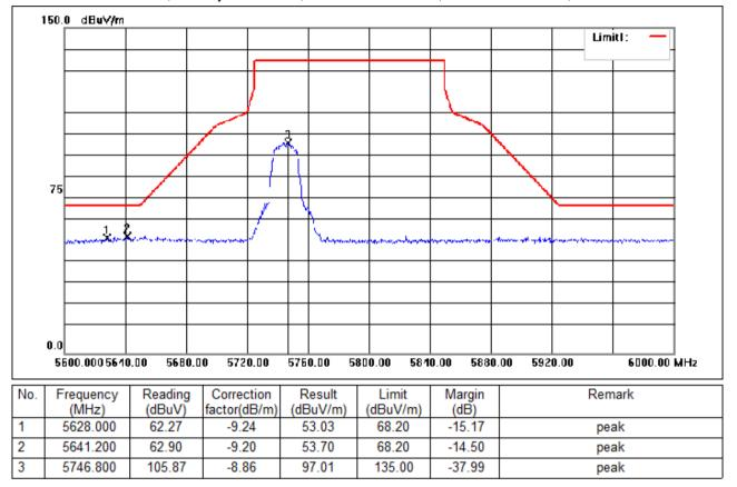
Test Mode: 04; Polarity: Horizontal; Modulation:802.11a; Bandwidth:20MHz; Channel:Low
