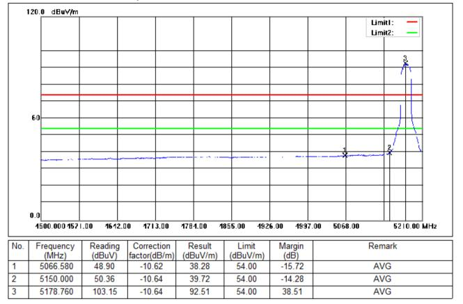
Test Mode: 01; Polarity: Horizontal; Modulation:802.11n; Bandwidth:20MHz; Channel:Low
