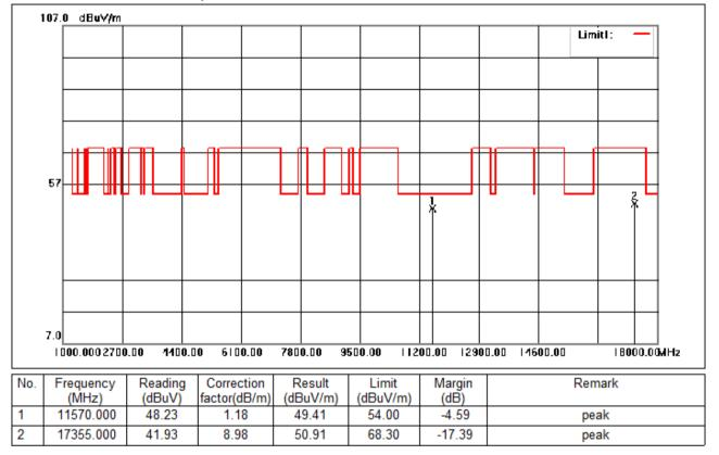
Test Mode: 04; Polarity: Horizontal; Modulation:802.11ac; Bandwidth:20MHz; Channel:middle
