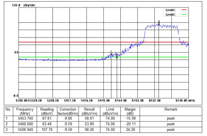
Test Mode: 03; Polarity: Horizontal; Modulation:802.11n; Bandwidth:40MHz; Channel:Low
