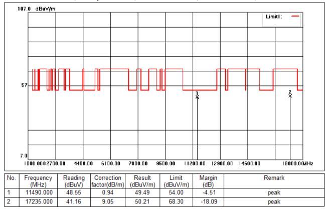
Test Mode: 04; Polarity: Horizontal; Modulation:802.11n; Bandwidth:20MHz; Channel:Low
