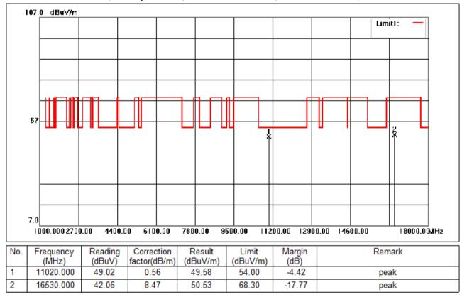
Test Mode: 03; Polarity: Vertical; Modulation:802.11ac; Bandwidth:40MHz; Channel:Low
