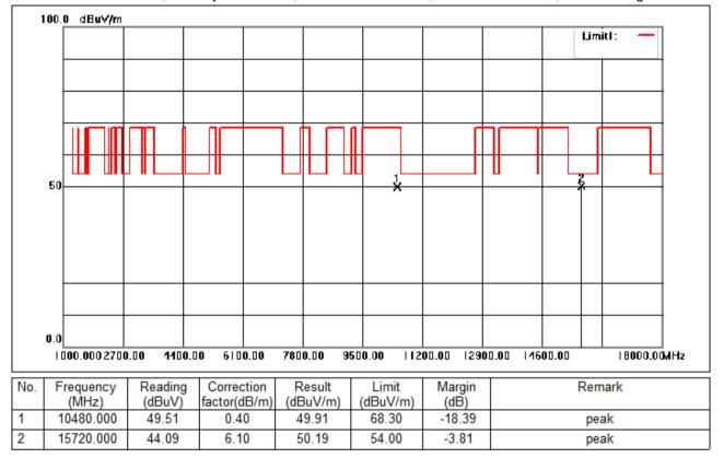
Test Mode: 01; Polarity: Horizontal; Modulation:802.11a; Bandwidth:20MHz; Channel:High
