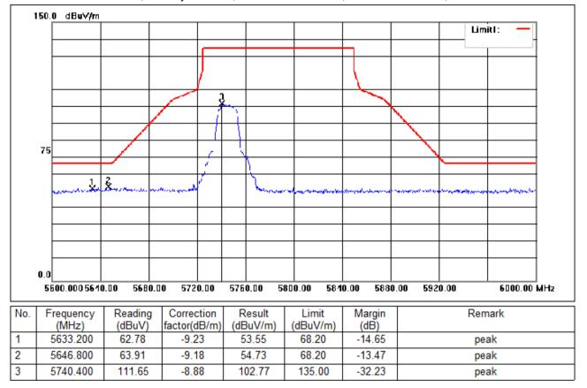
Test Mode: 04; Polarity: Vertical; Modulation:802.11a; Bandwidth:20MHz; Channel:Low
