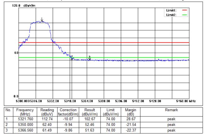
Test Mode: 02; Polarity: Horizontal; Modulation:802.11n; Bandwidth:20MHz; Channel:High
