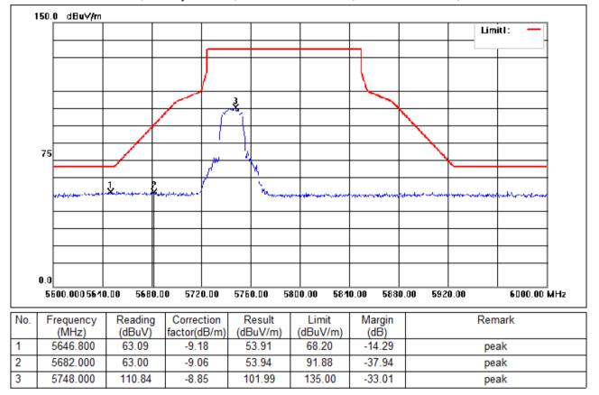
Test Mode: 04; Polarity: Vertical; Modulation:802.11ac; Bandwidth:20MHz; Channel:Low
