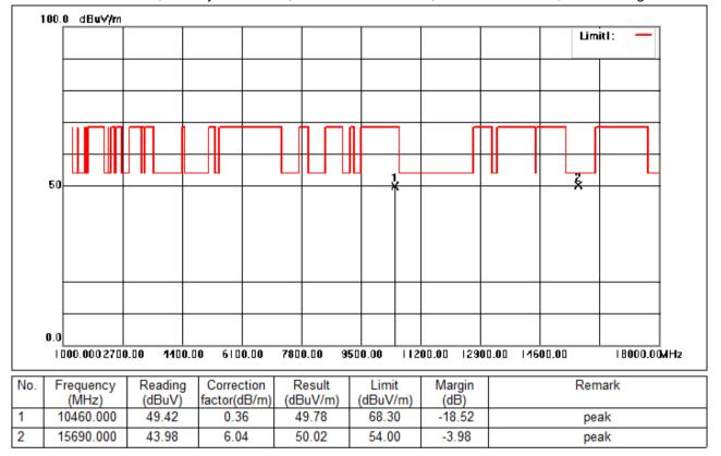
Test Mode: 01; Polarity: Horizontal; Modulation:802.11ac; Bandwidth:40MHz; Channel:High
