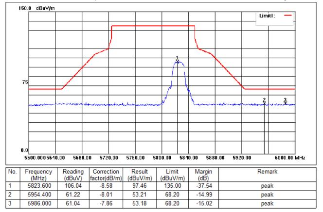
Test Mode: 04; Polarity: Horizontal; Modulation:802.11a; Bandwidth:20MHz; Channel:High
