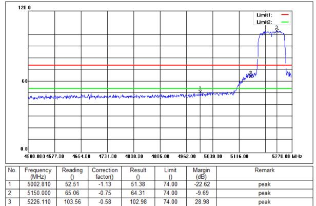
Mode:b; Polarization:Vertical; Modulation:c; bandwidth:80MHz; Channel:Low
