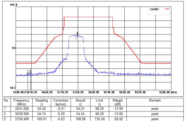
Mode:c; Polarization:Vertical; Modulation:c; bandwidth:40MHz; Channel:Low
