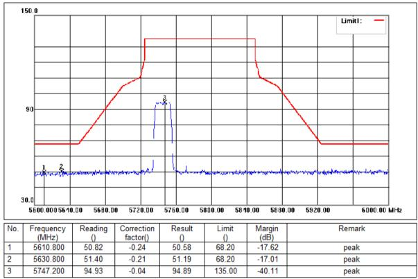
Mode:c; Polarization:Horizontal; Modulation:n; bandwidth:20MHz; Channel:Low
