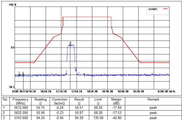
Mode:c; Polarization:Horizontal; Modulation:c; bandwidth:20MHz; Channel:Low
