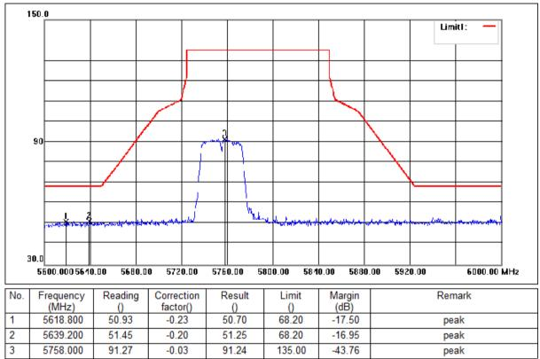
Mode:c; Polarization:Horizontal; Modulation:n; bandwidth:40MHz; Channel:Low
