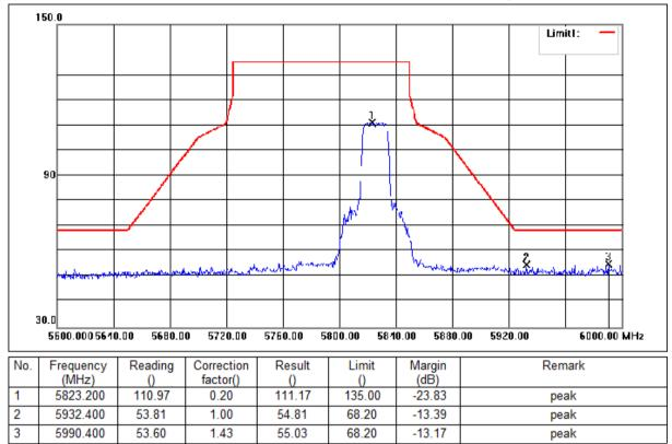
Mode:c; Polarization:Vertical; Modulation:a; bandwidth:20MHz; Channel:High
