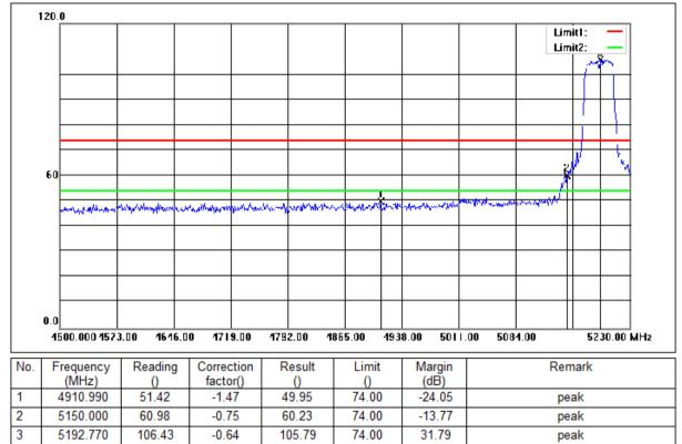
Mode:b; Polarization:Vertical; Modulation:n; bandwidth:40MHz; Channel:Low
