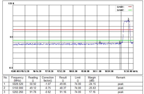
Mode:b; Polarization:Horizontal; Modulation:c; bandwidth:40MHz; Channel:Low
