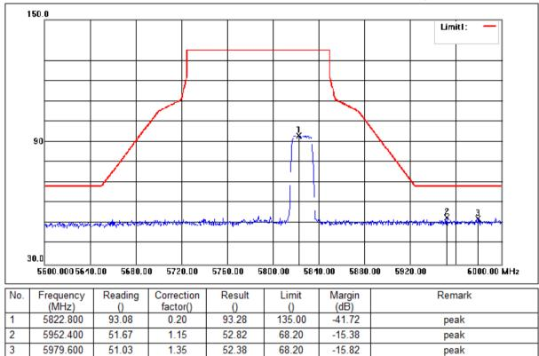
Mode:c; Polarization:Horizontal; Modulation:c; bandwidth:20MHz; Channel:High
