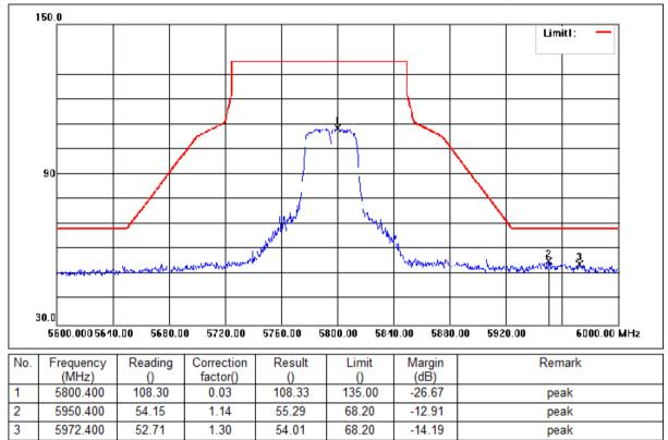
Mode:c; Polarization:Vertical; Modulation:n; bandwidth:40MHz; Channel:High
