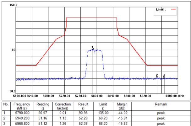
Mode:c; Polarization:Horizontal; Modulation:c; bandwidth:40MHz; Channel:High
