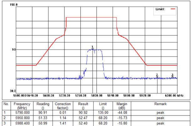
Mode:c; Polarization:Horizontal; Modulation:n; bandwidth:40MHz; Channel:High
