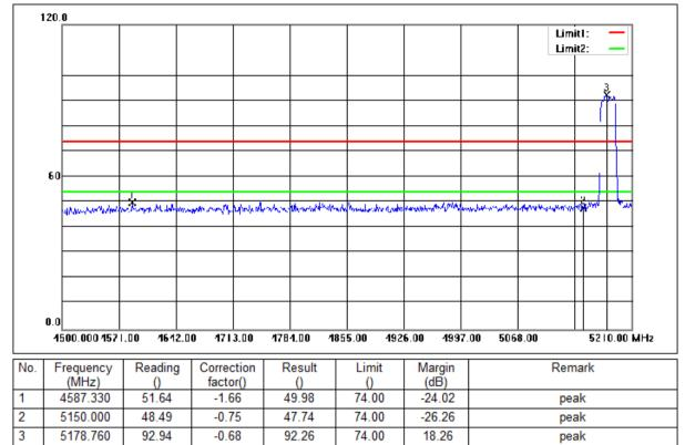
Mode:b; Polarization:Horizontal; Modulation:n; bandwidth:20MHz; Channel:Low
