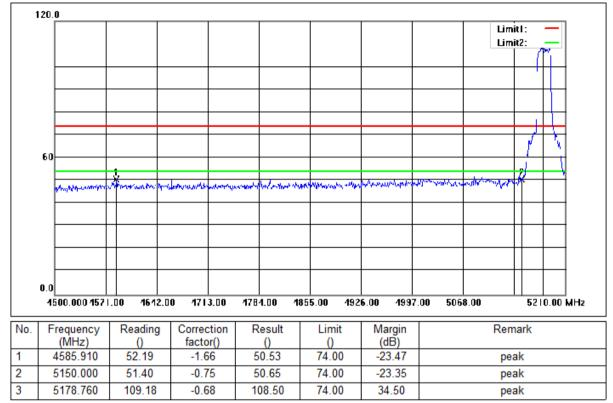
Mode:b; Polarization:Vertical; Modulation:a; bandwidth:20MHz; Channel:Low
