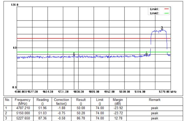
Mode:b; Polarization:Horizontal; Modulation:c; bandwidth:80MHz; Channel:Low
