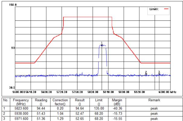
Mode:c; Polarization:Horizontal; Modulation:a; bandwidth:20MHz; Channel:High
