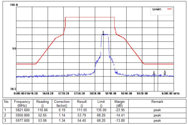
Mode:c; Polarization:Vertical; Modulation:n; bandwidth:20MHz; Channel:High
