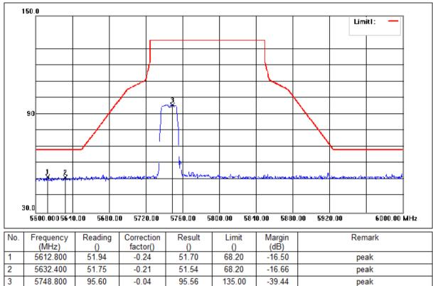
Mode:c; Polarization:Horizontal; Modulation:a; bandwidth:20MHz; Channel:Low
