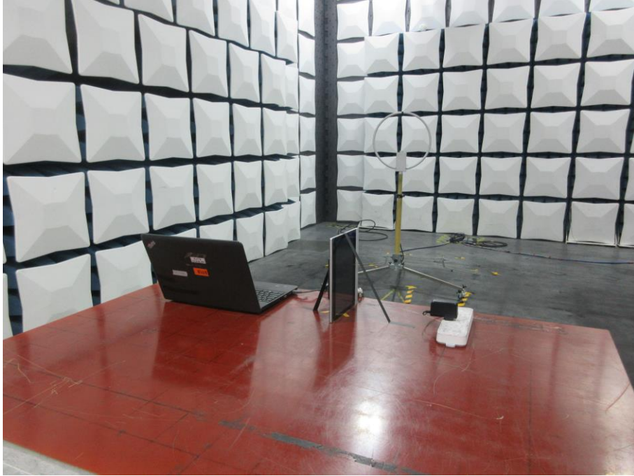
RADIATED RF MEASUREMENT SETUP (9KHz ~ 30 MHz)
