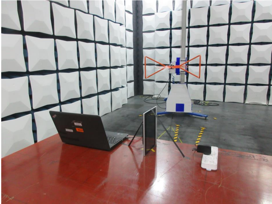
RADIATED RF MEASUREMENT SETUP (30MHz ~ 1 GHz)
