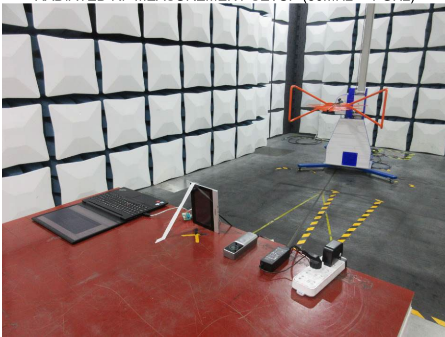
RADIATED RF MEASUREMENT SETUP (30MHz ~ 1 GHz)
