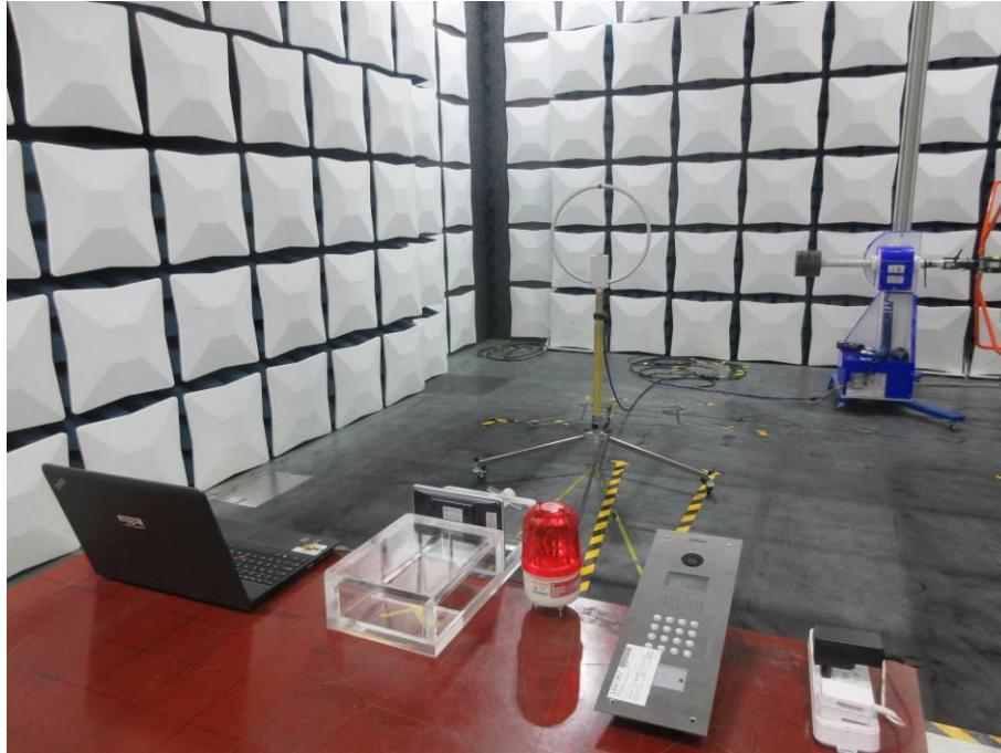
RADIATED RF MEASUREMENT SETUP (9KHz ~ 30 MHz)
