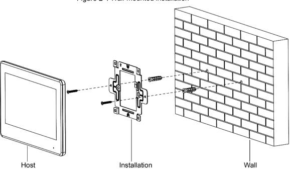
Figure 2-1 Wall-mounted installation
