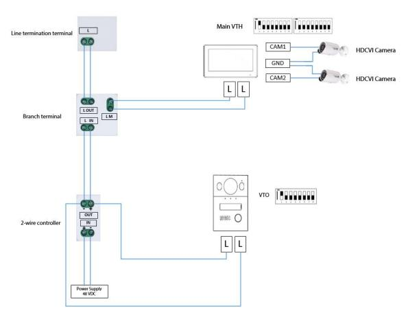
Wiring One VTO and Two VTH (cascade connection)
