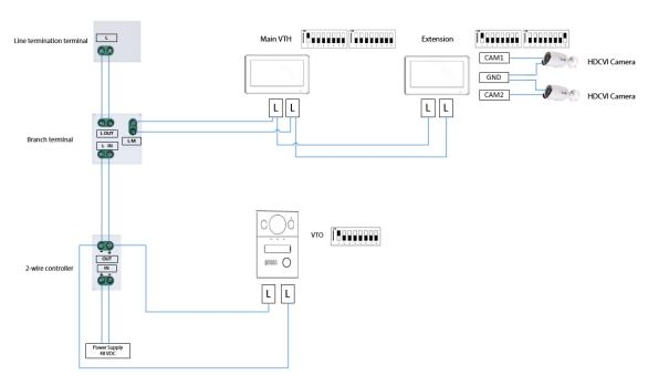
Wiring One VTO and Two VTH (parallel connection)
